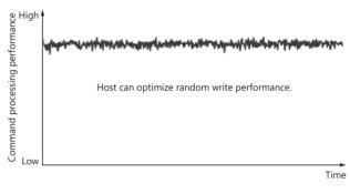
\*The number of SMR bands that can be accessed at once (maximum SMR band count) is stipulated in a specification. (This figure shows an example of command processing performance when a write command is executed to write fixed-size data of 4,096 bytes to 128 SMR bands.)
