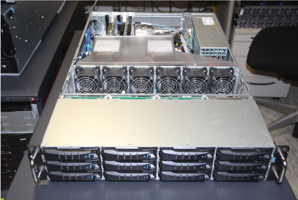
Picture 2: SB202-TU head node server from AIC
