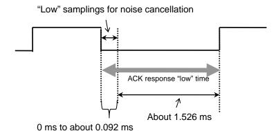
The "low" samplings for noise cancellation and the rising timing of data bit need to be configured the same. Values need to be carefully selected because the configuration of the rising timing of data bit affects "low" time of transmit data
