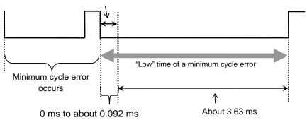
When a minimum cycle error occurs, "low" signal is output (about 3.63ms) after the elapse of "Low" samplings for noise cancellation.
