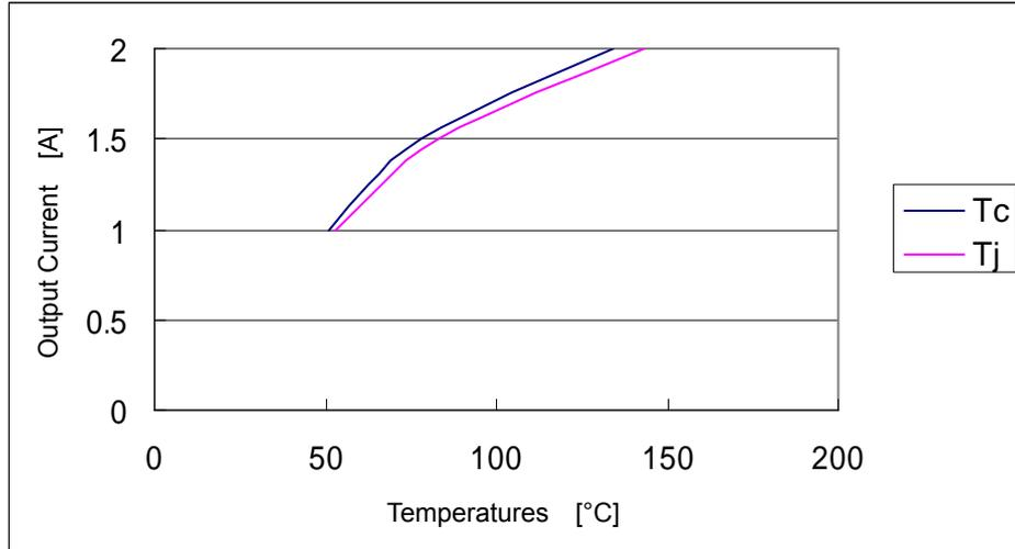
Conditions:  $T_a = 25^\circ\text{C}$  VM = 24 V IN2, PWM, RSGND = GND, TISD, VISD; 20 k  $\Omega$ , OSC = GND IN1 =  $-100 \mu\text{A}$  (Diode voltage monitor circuit), on a PCB
