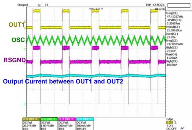
Reference waveforms when VREF = 2.0 V
