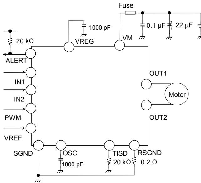
**Application Circuit Example When NOT Using Constant Current PWM Control**
