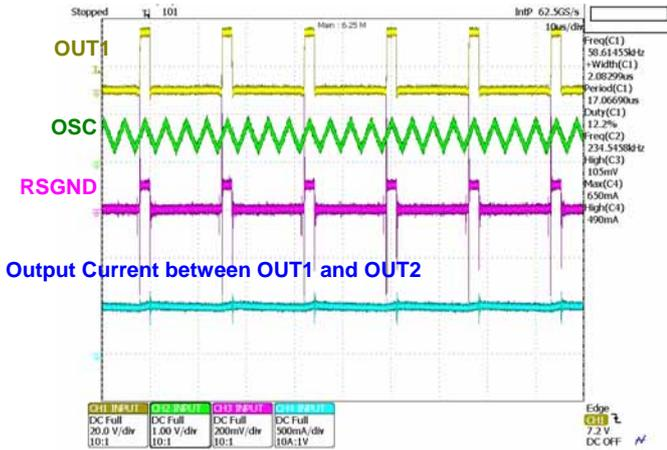
Reference waveforms when VREF = 0 V
