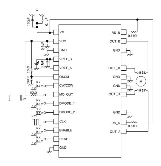
Note: Bypass capacitors should be added as necessary.
