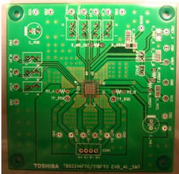
【Glass-epoxy four-layer board for QFN48-P-0707-0.5】
