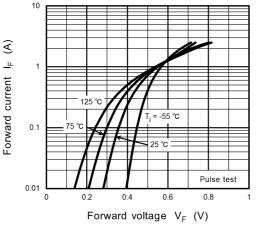
Fig. 10.1 I<sub>F</sub> - V<sub>F</sub> (Reference Maximum)
