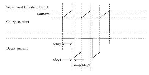
Figure 7.1 Constant current PWM waveform timing chart example 2
