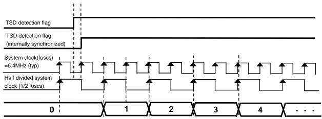
Figure 6.2 Dead band time of over thermal detection
