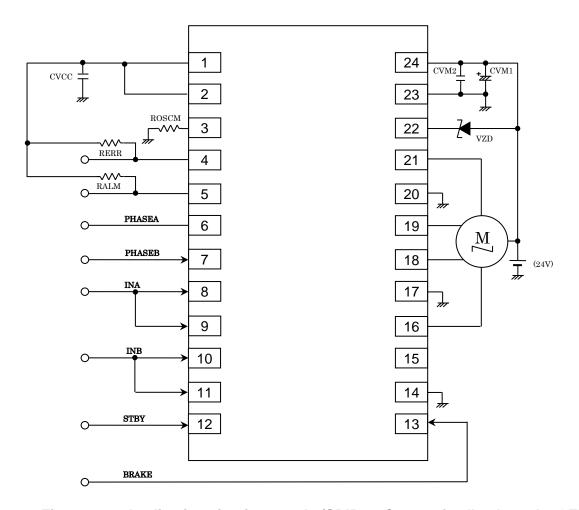
Figure 9.4 Application circuit example (SDIP24\_Current feedback mode: OFF)
