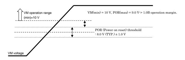
Figure 1.1 Power supply voltage and operation range
