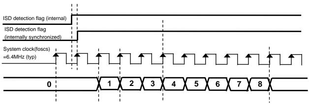
Figure 6.1 Dead band time of over current detection
