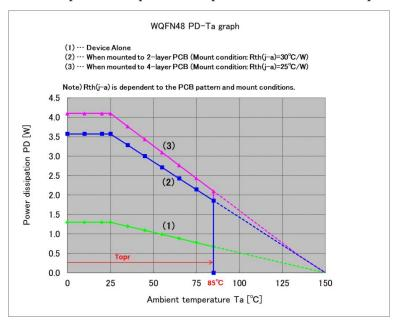
Figure 8.1 Power dissipation (WQFN48)
