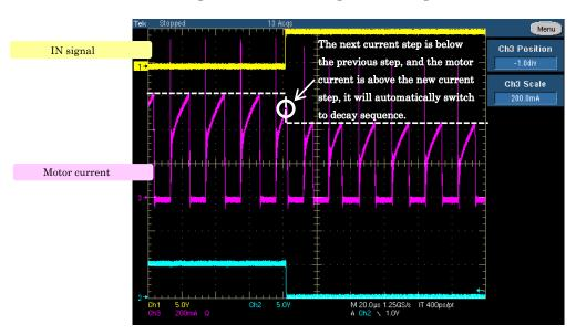
Figure 4.3 Constant current PWM waveform(next step is lower than previous)
