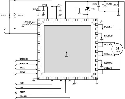
Figure 9.1 Application circuit example (Current feedback mode: ON)
