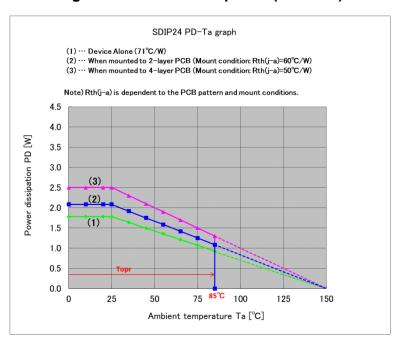
Figure 8.2 Power dissipation (SDIP24)
