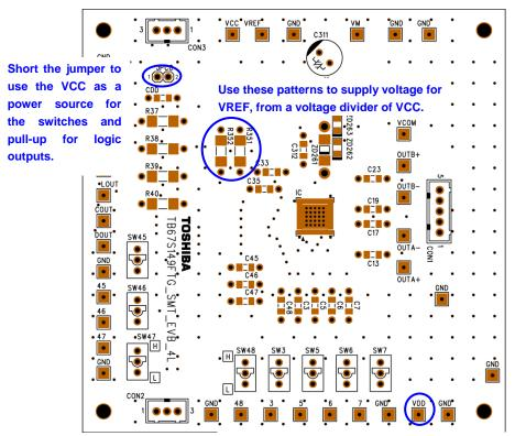
To use another power source for switches and logic outputs, supply a voltage to the VDD pin. While using the VDD pin you must keep the JPCC (jumper in the upper left) open.
