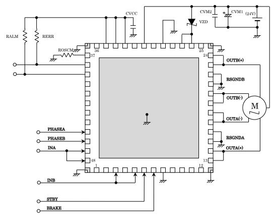
Figure 9.2 Application circuit example (WQFN48\_Current feedback mode: OFF)
