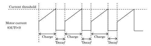
Figure 4.1 Constant current PWM timing chart 1
