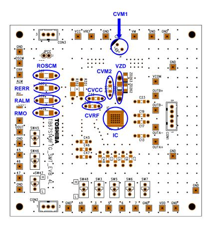
Figure 10.2 Main parts(WQFN48)
