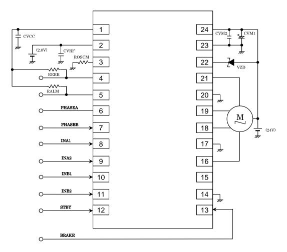
Figure 9.3 Application circuit example (SDIP24\_Current feedback mode: ON)
