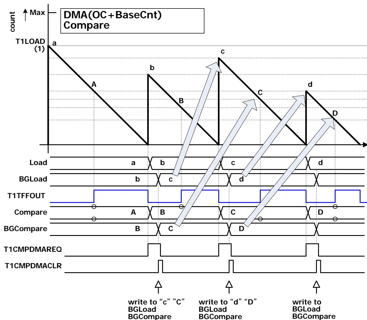
Figure 5.25 DMA (output comparison and base counter) operation
