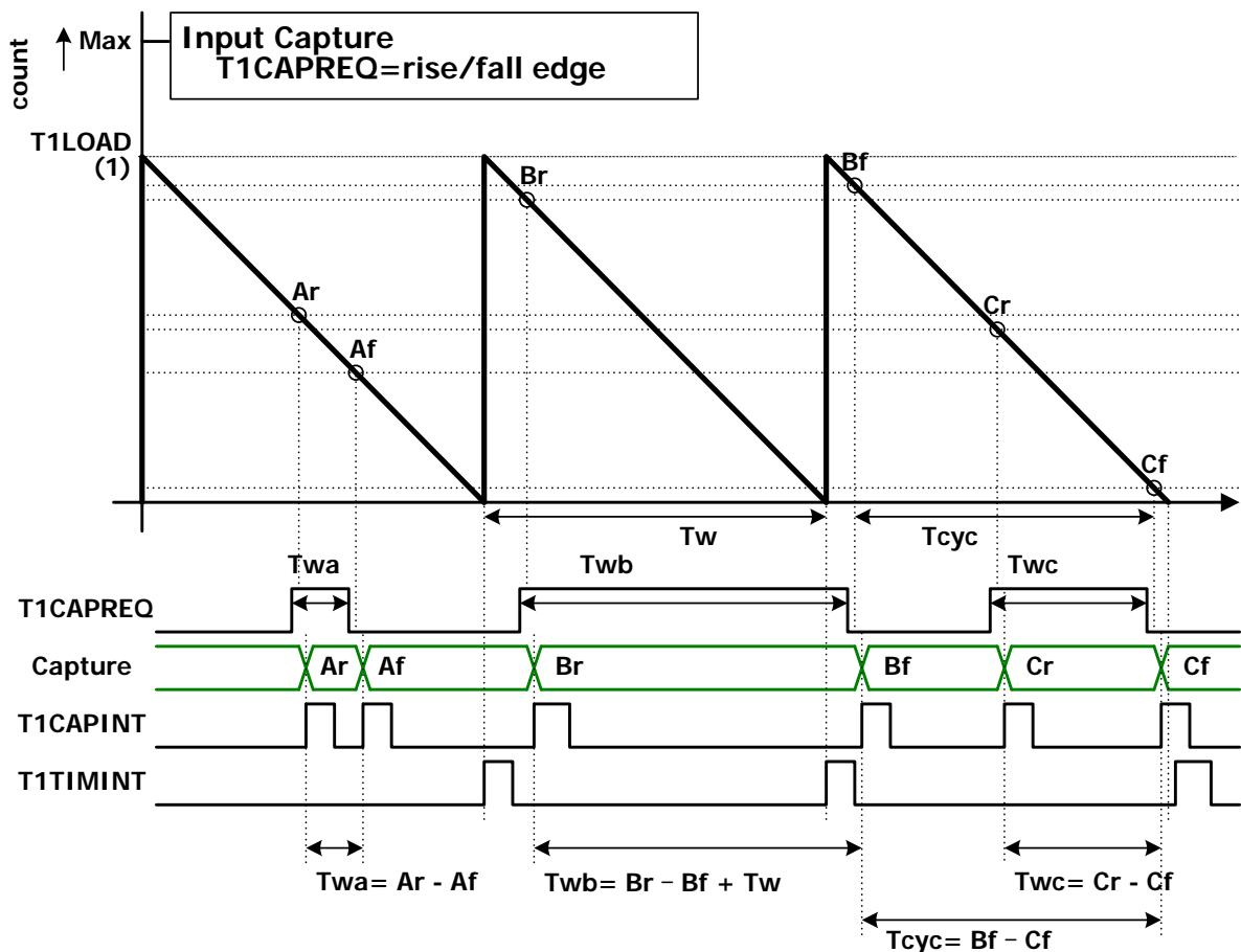
Figure 5.12 Input capture PWM operation (One channel)
