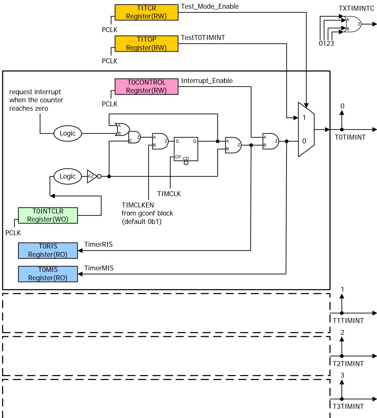
Figure 5.28 Outline diagram of interrupt generator
