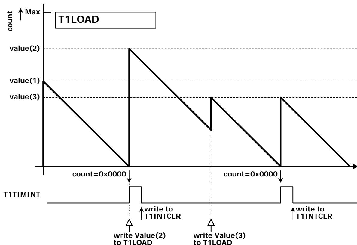
Figure 5.8 Load Register Change Operation
