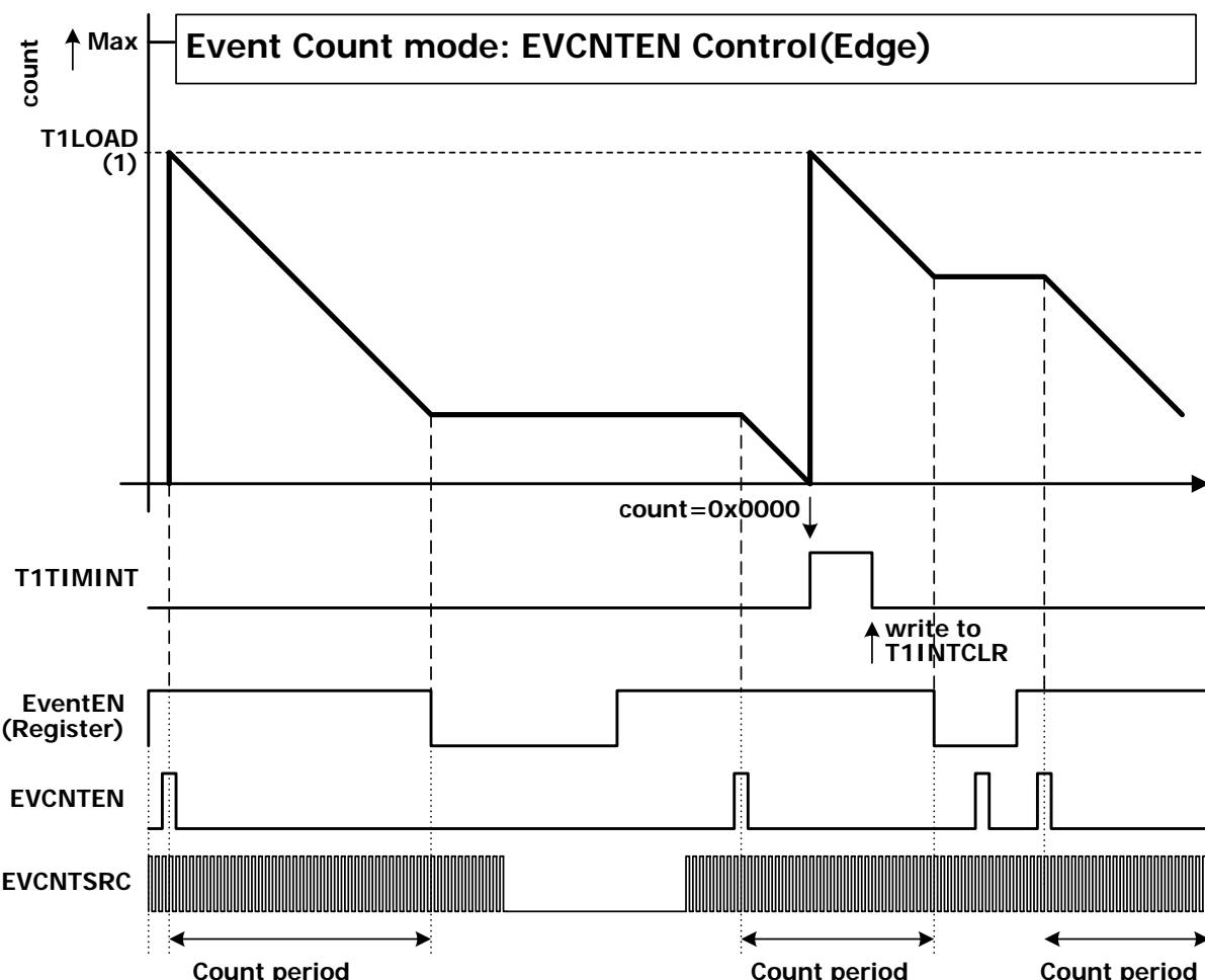
Figure 5.20 Event counter operation (EVCNTEN pin control: edge)
