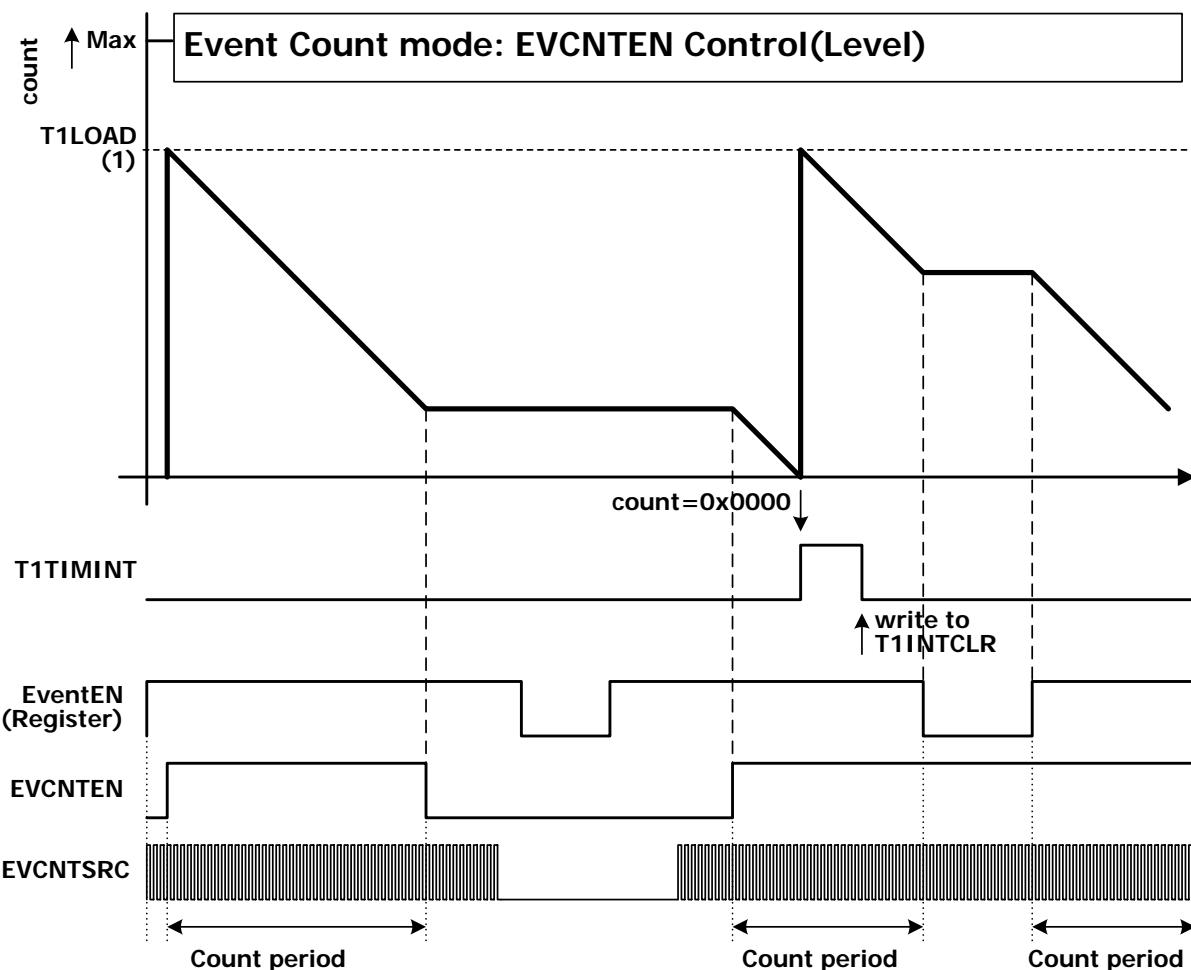
Figure 5.19 Event counter operation (EVCNTEN pin control: Level)
