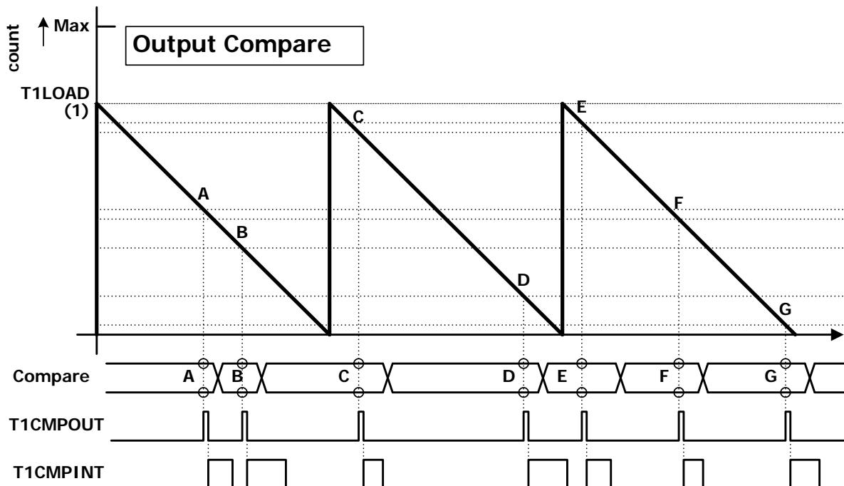
Figure 5.14 Output comparison operation (One channel)
