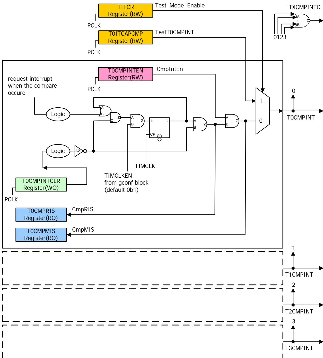
Figure 5.30 Outline diagram of comparison interrupt generator
