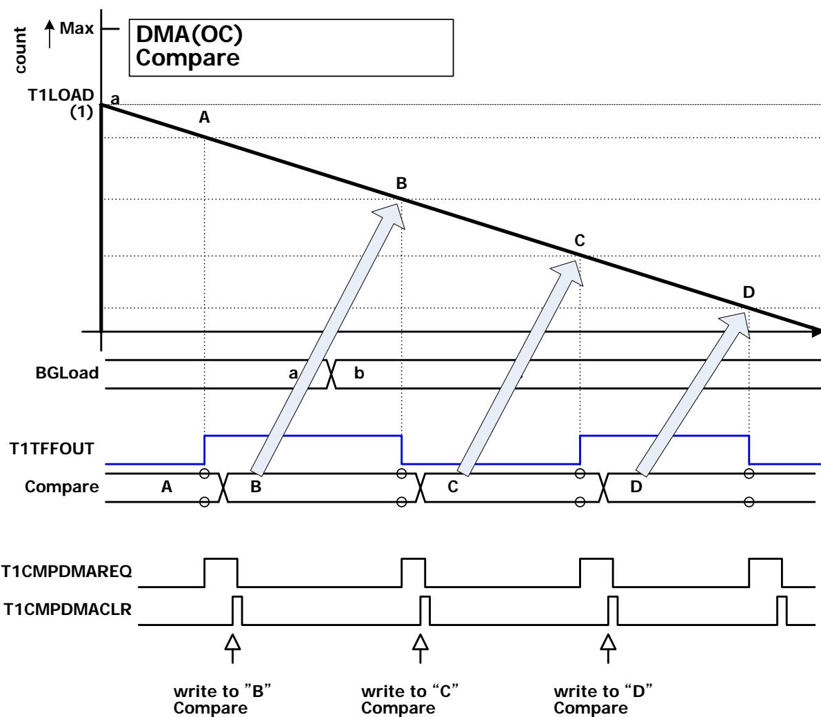
**Figure 5.24 DMA (output compare) operation**
