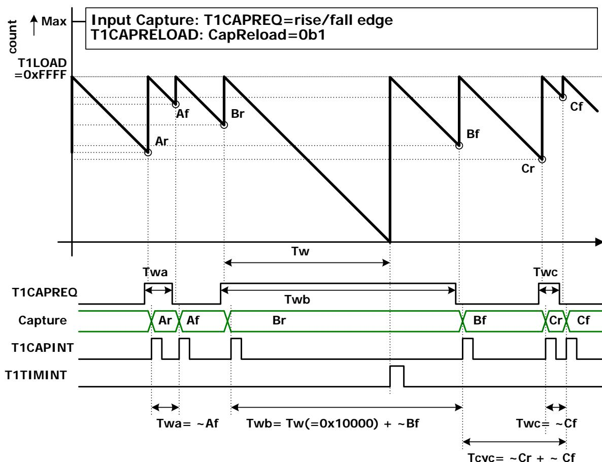
Figure 5.13 Input capture PWM operation (Reload)
