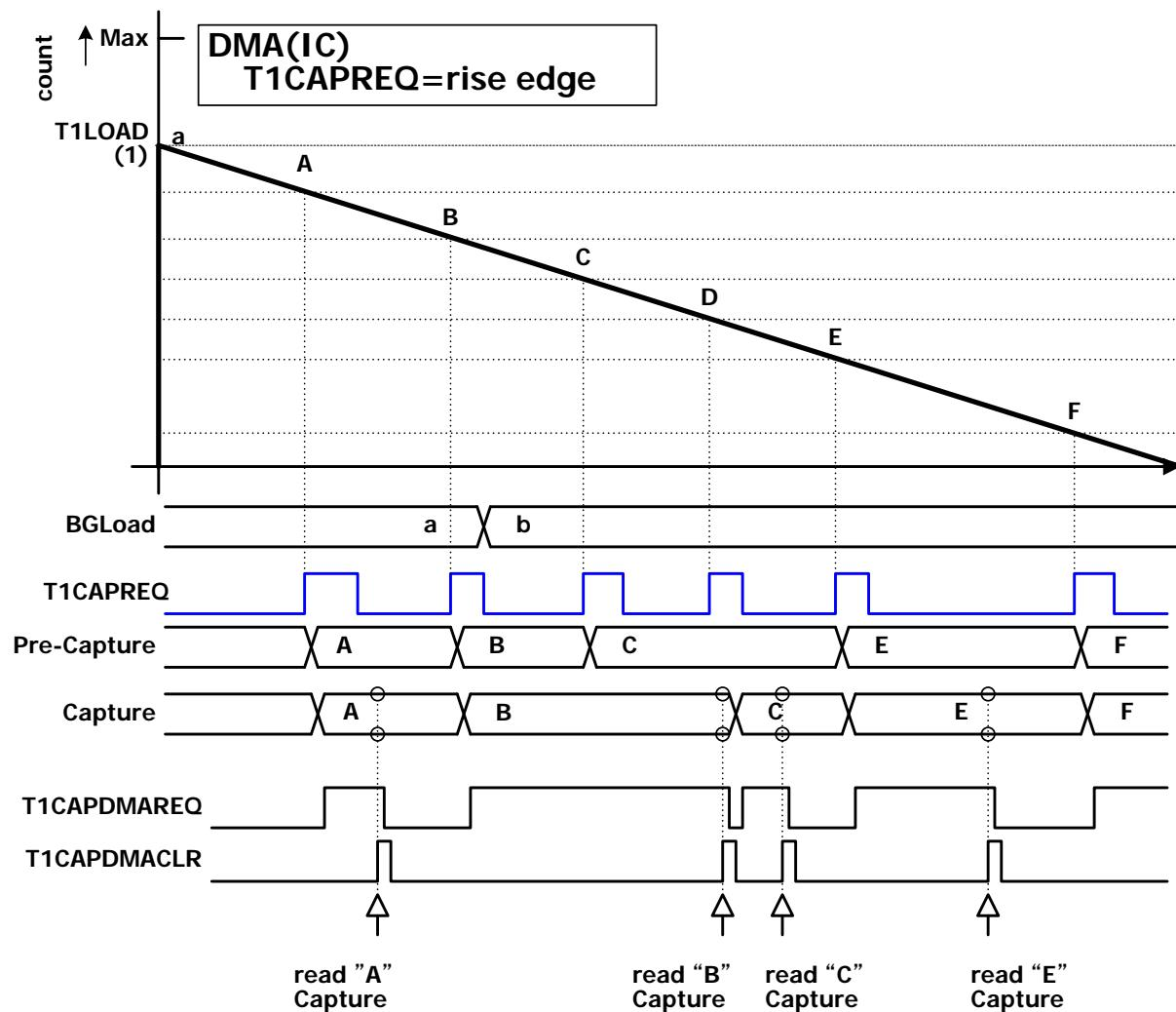
Figure 5.23 DMA (input capture) operation
