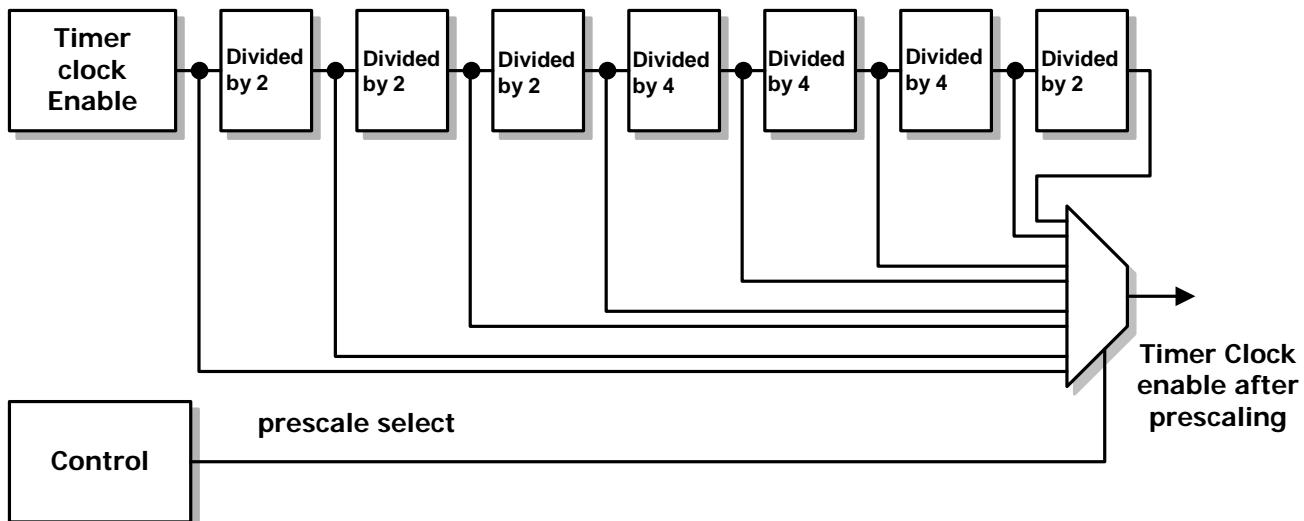
Figure 5.3 Block diagram of Prescaler
