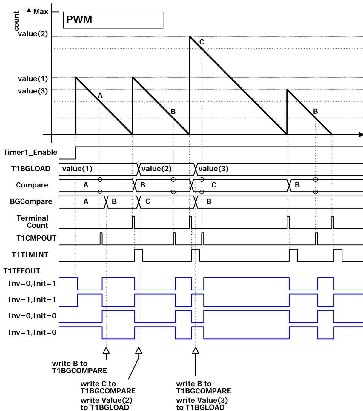
Figure 5.17 Output comparison PWM Operation (2)
