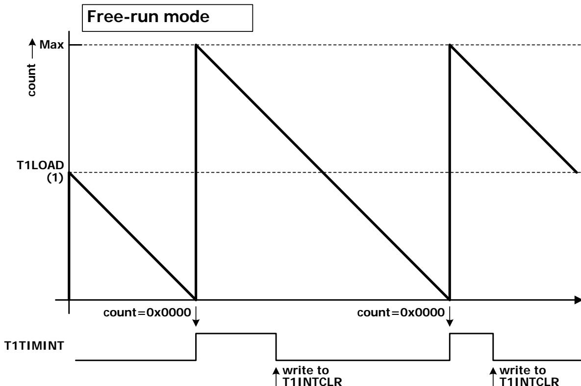
Figure 5.7 Free-run timer wrapping mode
