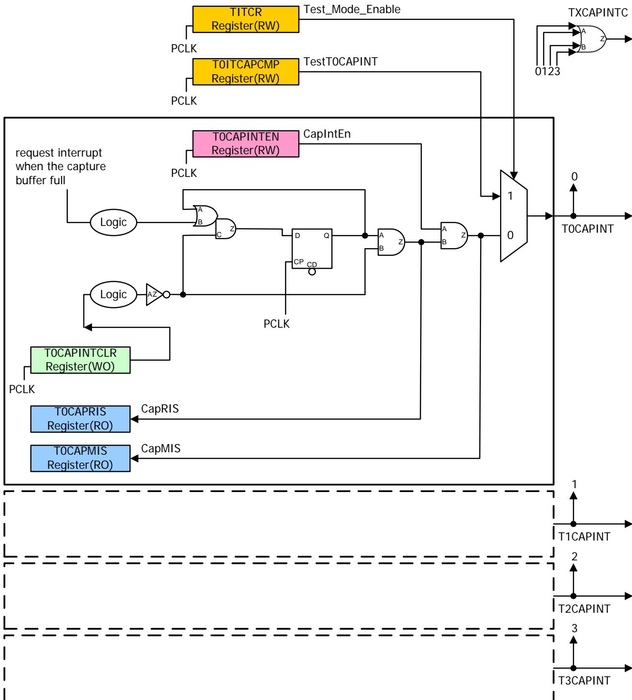
Figure 5.29 Outline diagram of capture interrupt generator
