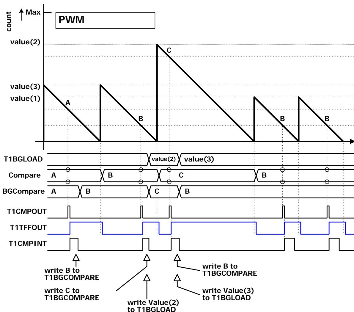
Figure 5.16 Output comparison PWM operation (1)
