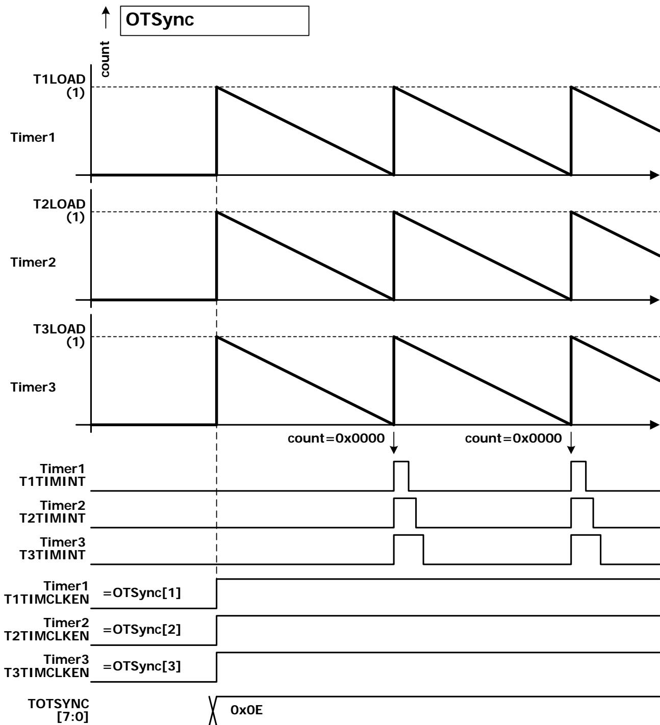
Figure 5.22 Count synchronization operation
