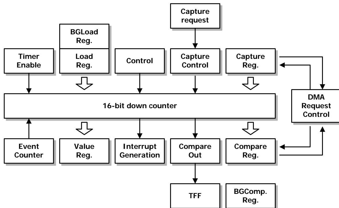
Figure 2.2 1 channel block diagram of ADVTMR
