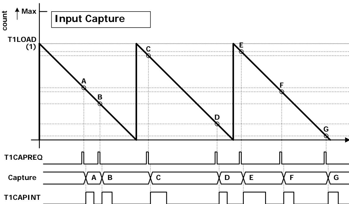
Figure 5.10 Input capture operation (One channel)
