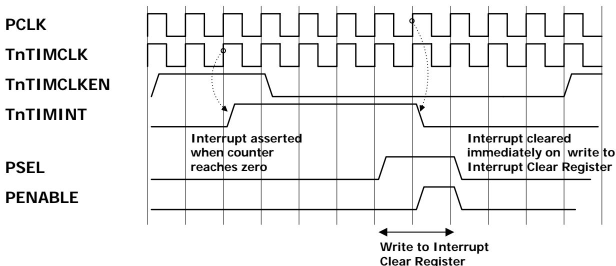
Figure 5.27 Example of interrupt generation
