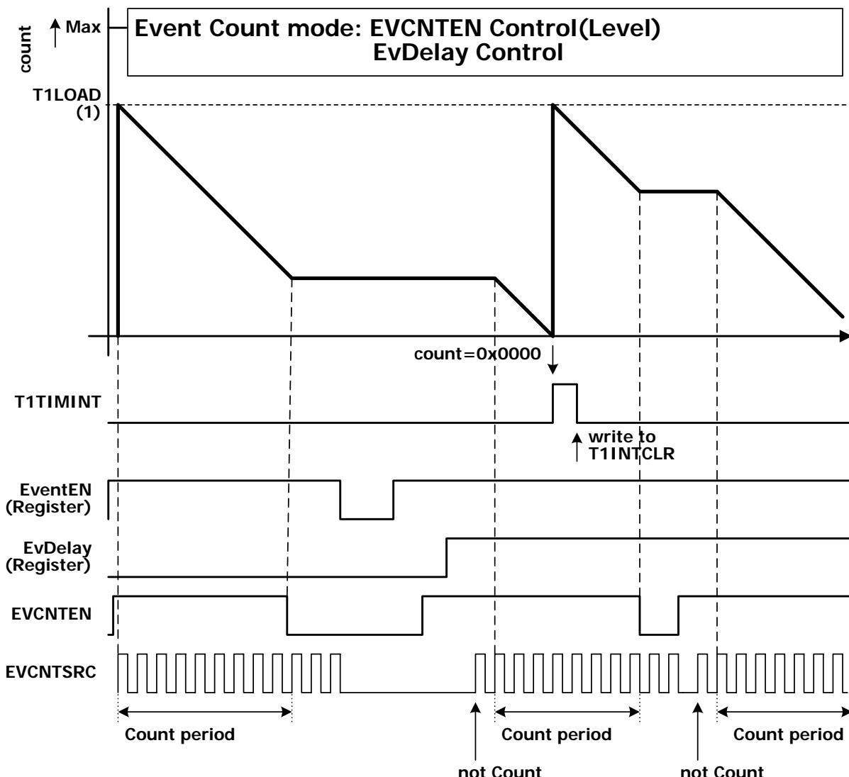
Figure 5.21 Event counter operation (EvDelay bit control)
