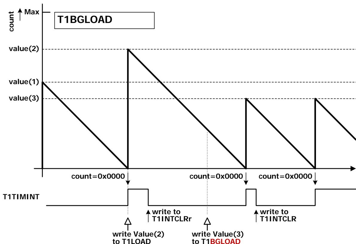
Figure 5.9 Background load register change operation
