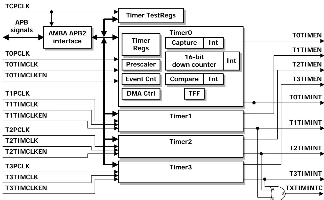
Figure 2.1 ADVTMR internal block diagram
