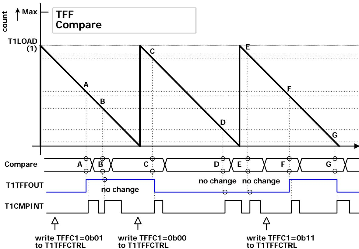
Figure 5.15 Output comparison TFF control (One channel)
