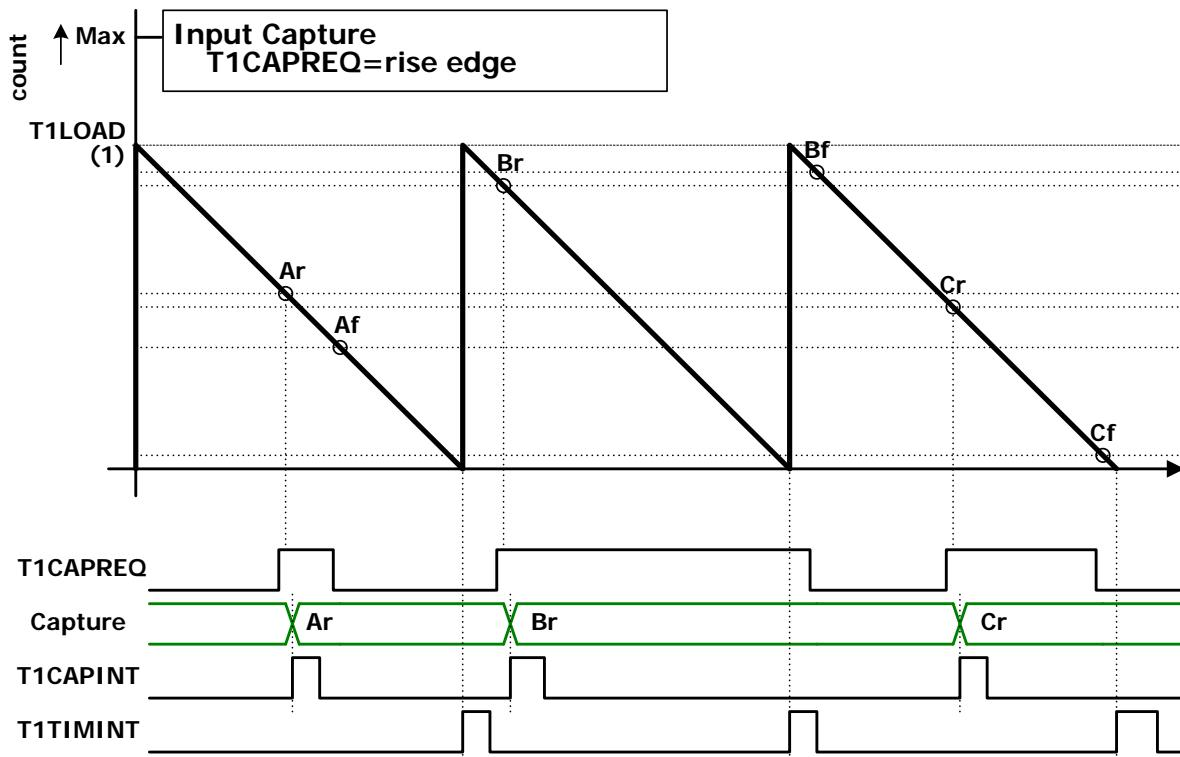
Figure 5.11 Input capture edge control
