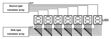
•Construction of output circuit
