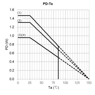
(1)APG type alone (2)When mounted on AFWG type (75  $\times$  114  $\times$  1.6 mm Cu 20%, single-side glass epoxy) (3)When mounted on AFNG type (50  $\times$  50  $\times$  1.6 mm Cu 40%, single-side glass epoxy) (4)AFG type alone
