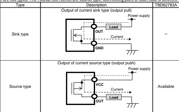
Dynamic drive control is possible by combining transistor arrays of the sink type and the source type.
