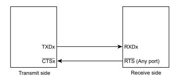
Figure 13-11 Handshake Function
