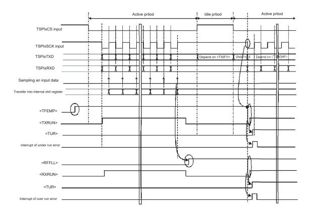
Figure 15-17 Overrun error and under run error
