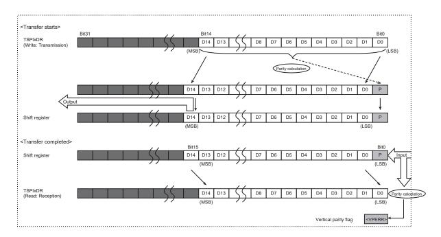
Figure 15-8 MSB first (15 bits data with parity)
