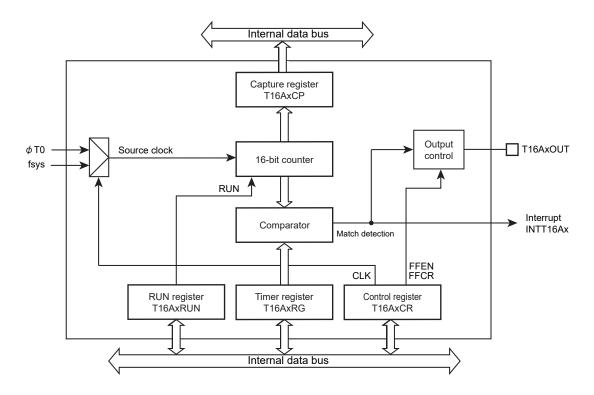
Figure 11-1 Block diagram of TMR16A
