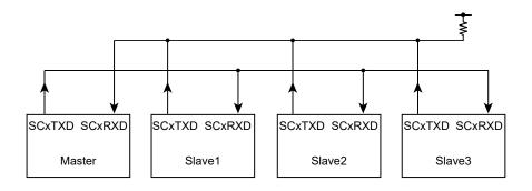
Figure 13-21 Serial Links to Use Wake-up Function
