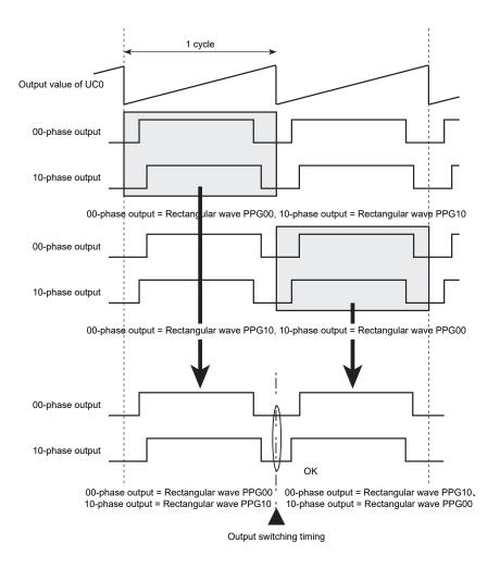
Figure 12-20 Waves before/after phase advance/delay (output SW) (A trailing edge of rectangular wave PPG10 is within UC0 cycle.)
