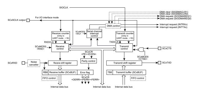
Figure 13-1 Serial Channel Block Diagram
