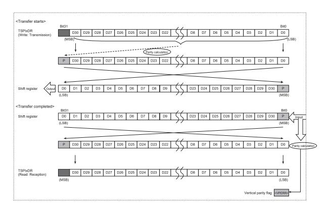
Figure 15-9 LSB first (31 bits data with parity)
