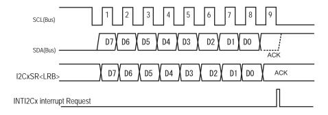
Figure 14-15 Last Received Bit Monitor
