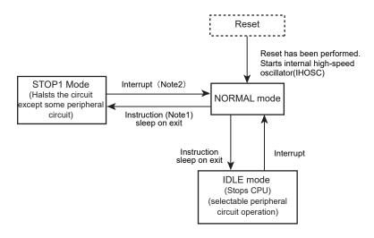
Figure 6-2 Mode Transition Diagram
