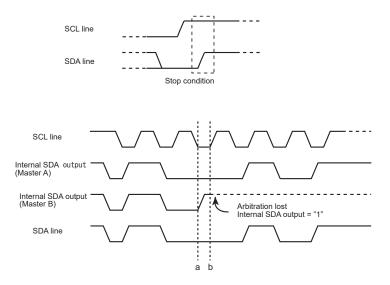
Figure 14-9 Generating the Stop Condition
