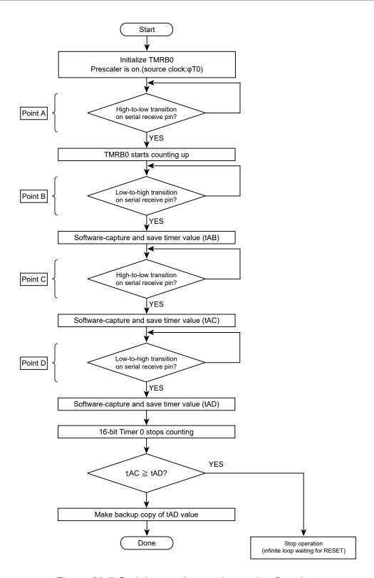
Figure 20-7 Serial operation mode receive flowchart
