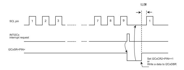
Figure 14-10 I2CxSR<PIN> and SCL
