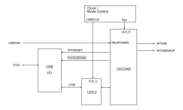
Figure 16-16 Connection Diagram of Power Management Control Signal
