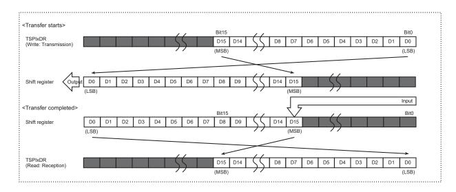
Figure 15-6 LSB first (16-bit data without a parity bit)
