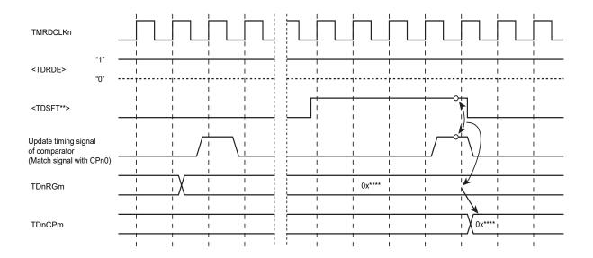
Figure 12-10 Update timing of CPn0,CPn1,CPn2 in PPG mode (<TDMDCY\*\*[2:0]> = "000")
