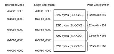
Figure 20-1 Block configuration
