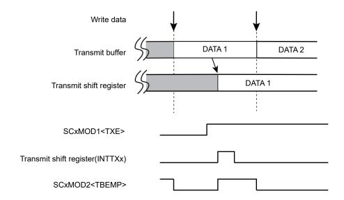
Figure 13-8 Operation of Transmit Buffer (Double-buffer is enabled)
