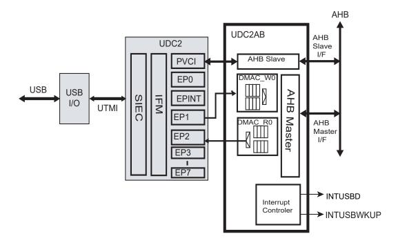
Figure 16-2 UDC2AB Block Diagram
