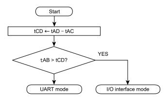
Figure 20-8 Serial operation mode determination flowchart
