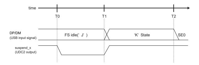
Figure 16-29 Resume operation timing by the host
