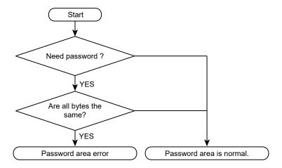
Figure 20-10 Password area check flowchart
