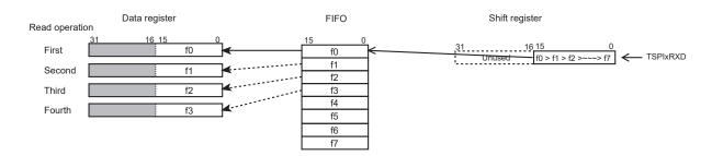
Figure 15-14 Operation in 7- to 16-bit data length
