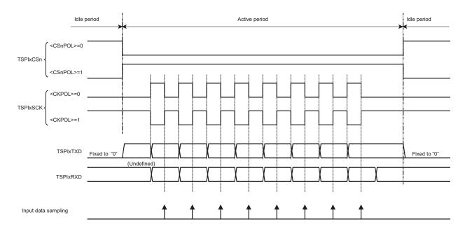
Figure 15-12 Idle period in SPI mode and the transmit pin status
