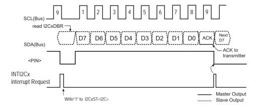
Figure 14-19 I2CxCR1<BC[2:0]>= 000,I2CxCR1<ACK>= 1 (Receiver Mode)
