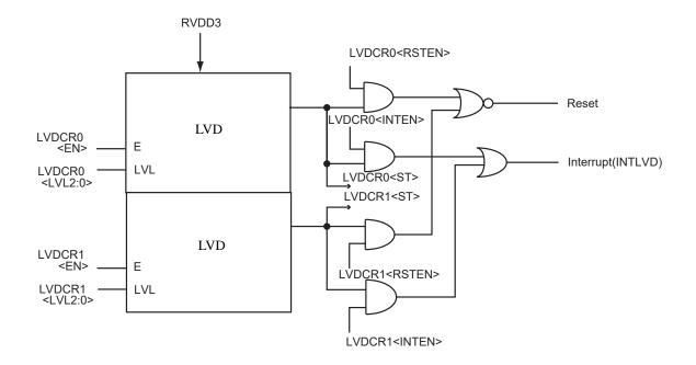
Figure 18-1 LVD Block Diagram
