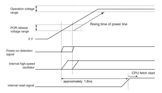
Figure 5-2 Cold reset with power-on-circuit
