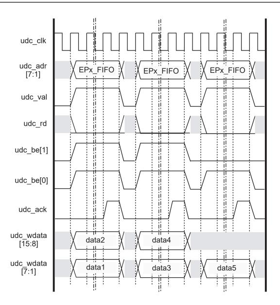
Figure 16-31 MPS write access with max pkt = odd number (common bus access)
