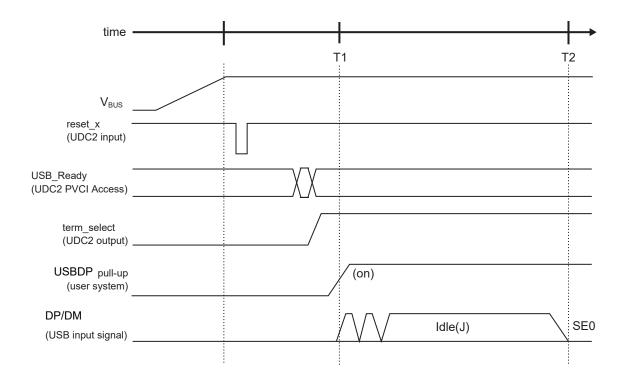
Figure 16-26 Connect operation timing
