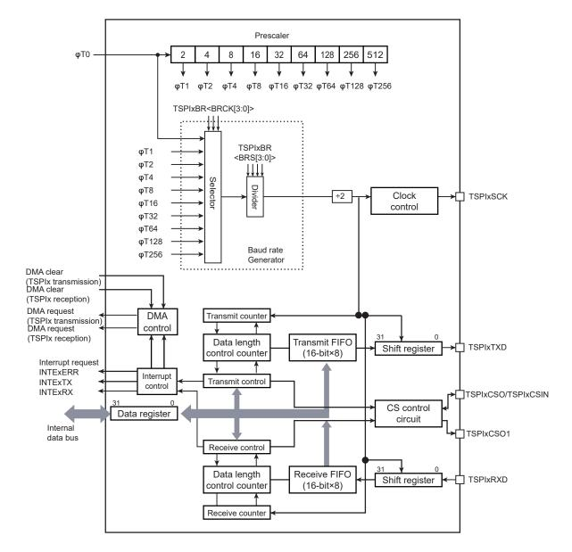
Figure 15-1 Block diagram of TSPIx
