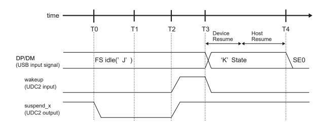
Figure 16-30 Remote wakeup operation timing
