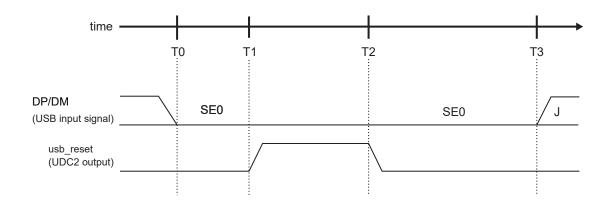
Figure 16-27 Reset Operation Timing
