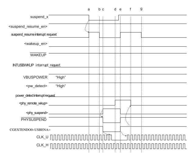
Figure 16-20 Operation of suspend/remote wakeup signals
