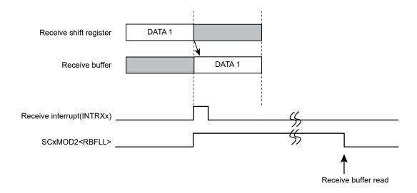
Figure 13-5 Receive Buffer Operation
