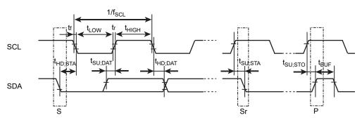
S: Start condition Sr: Repeated-start condition P: Stop condition
