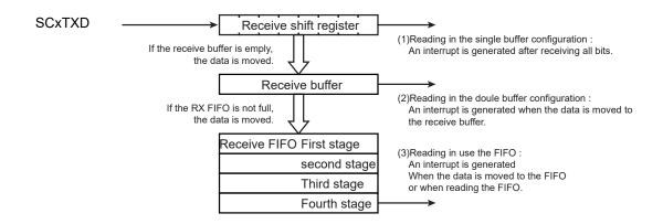
Figure 13-13 Receive Buffer/FIFO Configuration Diagram
