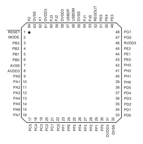
Figure 1-2 Pin Layout (LQFP64 TOP VIEW)
