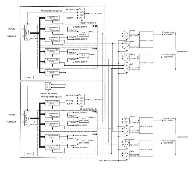
Figure 12-1 Block diagram of TMRD timer unit
