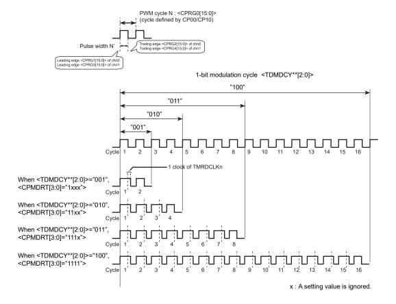
Figure 12-9 Schematic diagram of 1-bit modulation function
