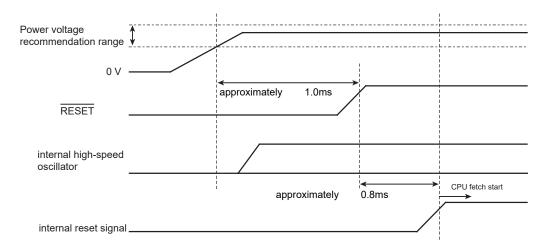
Figure 5-1 Cold reset Operation Sequence
