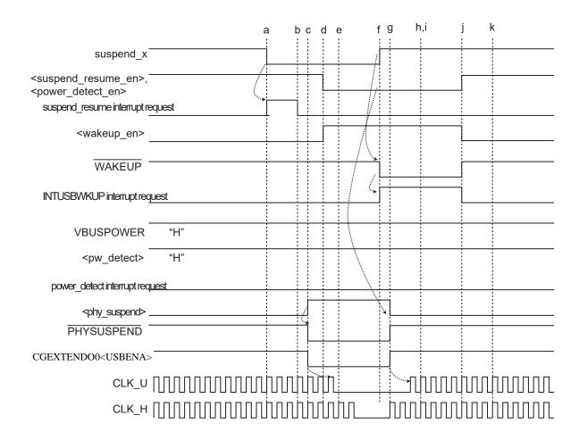
Figure 16-17 Signal operations when suspended and resumed (when CLK H is stopped)
