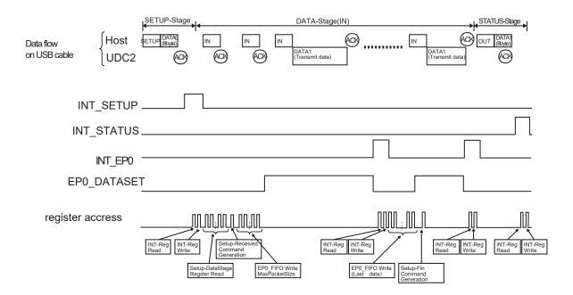
Figure 16-22 Flow of the control in Control-RD transfer
