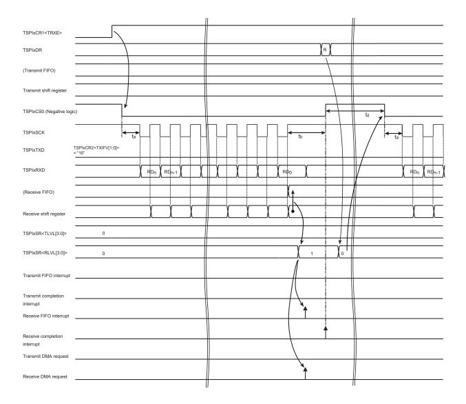
Figure 15-20 Operation example in receive mode
