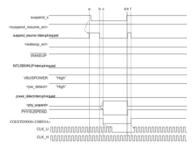
Figure 16-18 Operation of suspend/resume signals (to get the CLK H work)
