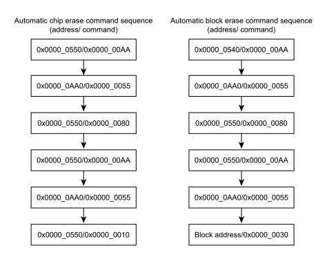
Figure 20-5 Flowchart of automatic erase
