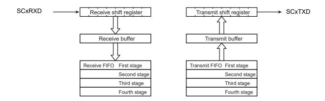
Figure 13-4 The Configuration of Buffer and FIFO
