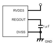
Figure 1-5 Capacitor connection of Regulator
