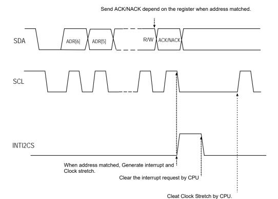
Figure 14-26 Address match Wake-up Function
