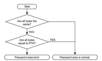
Figure 20-9 Password area check flowchart
