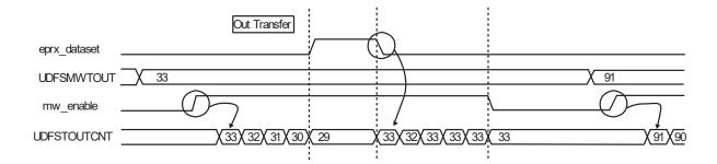
Figure 16-15 Example of MW timeout count
