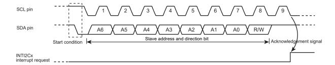
Figure 14-8 Generating the Start Condition and a Slave Address
