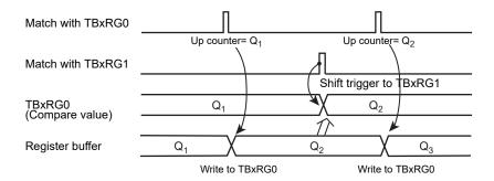
Figure 10-3 Register buffer operation
