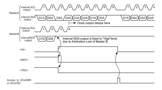
Figure 14-12 Example of Master B Lost Arbitration (D7A = D7B, D6A = D6B)
