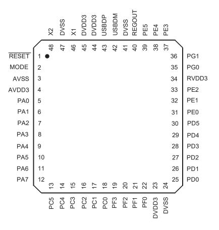
Figure 1-3 QFN48 TOP VIEW
