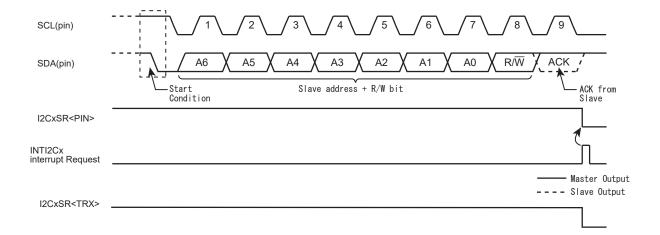
Figure 14-17 Generating the Start Condition and a Slave Address
