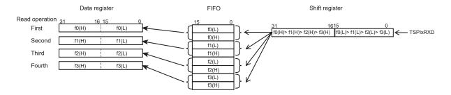
Figure 15-15 Operation in 17- to 32-bit data length
