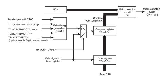
Figure 12-5 Configuration of comparator (CP05)
