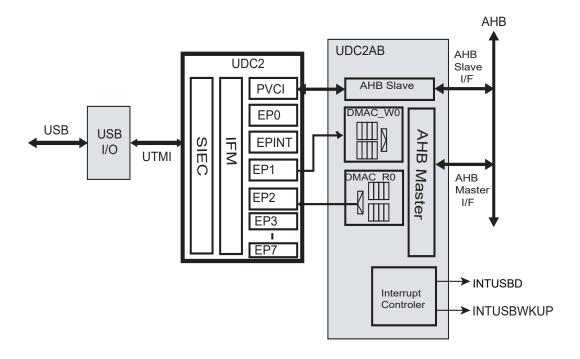
Figure 16-5 Block diagram of UDC2
