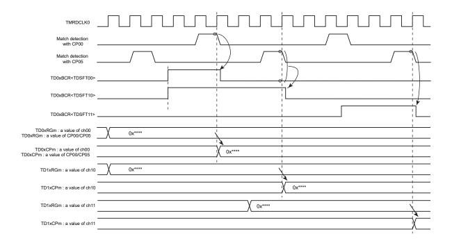
Figure 12-18 A timing to set update enable register is delayed than a match with CP05
