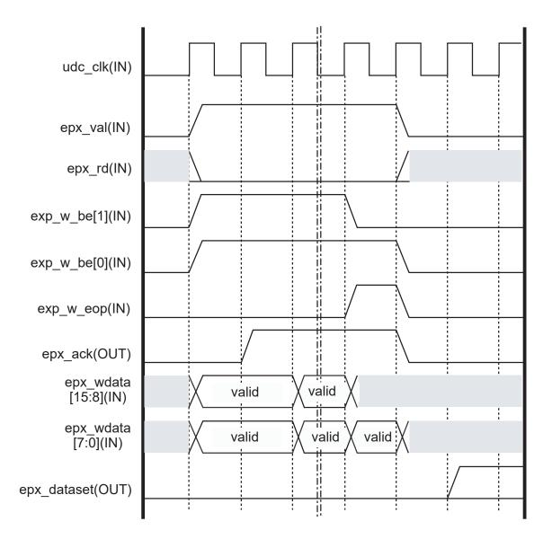
Figure 16-32 MPS (odd number) write access with max\_pkt = even number (EP direct access)
