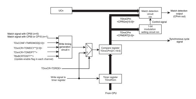
Figure 12-3 Configuration of comparators (CP02, CP04, CP12, CP14)
