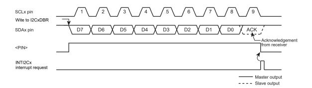
Figure 14-18 <BC[2:0]>= 000,<ACK>= 1 (Transmitter Mode)
