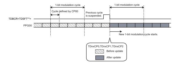
Figure 12-13 Update timing of 1-bit modulation in PPG mode
