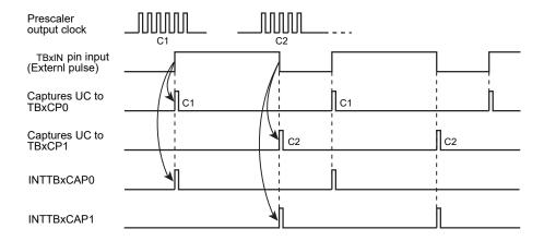
Figure 10-7 Pulse width measurement
