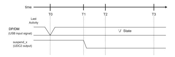
Figure 16-28 Suspend operation timing
