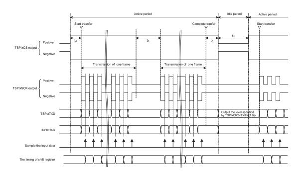
Figure 15-11 Transfer format and timing adjustment
