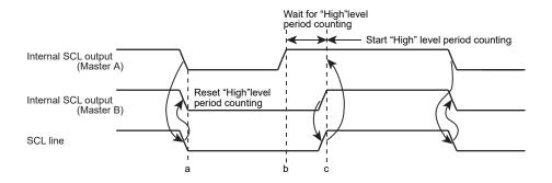
Figure 14-7 Example of Clock Synchronization
