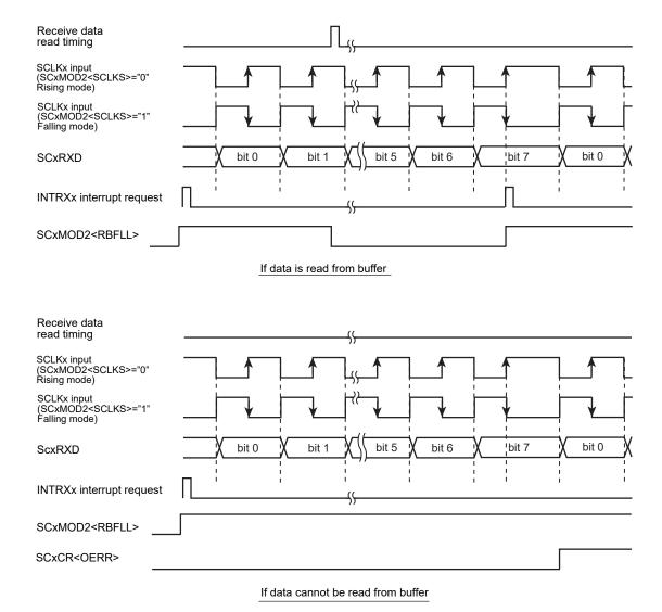
Figure 13-18 Receive Operation in the I/O Interface Mode (Clock Input Mode)
