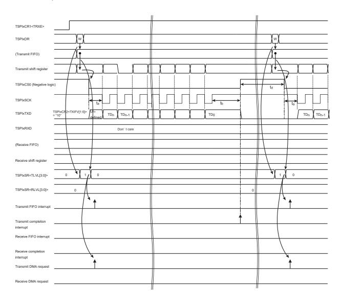
Figure 15-19 Operation example of transmit mode
