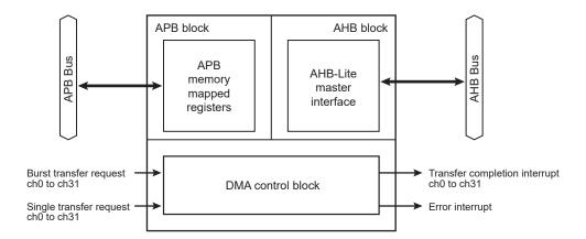
Figure 8-1 µDMA block diagram
