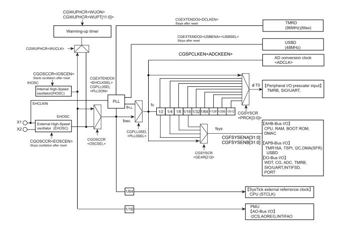
Figure 6-1 Clock Block Diagram
