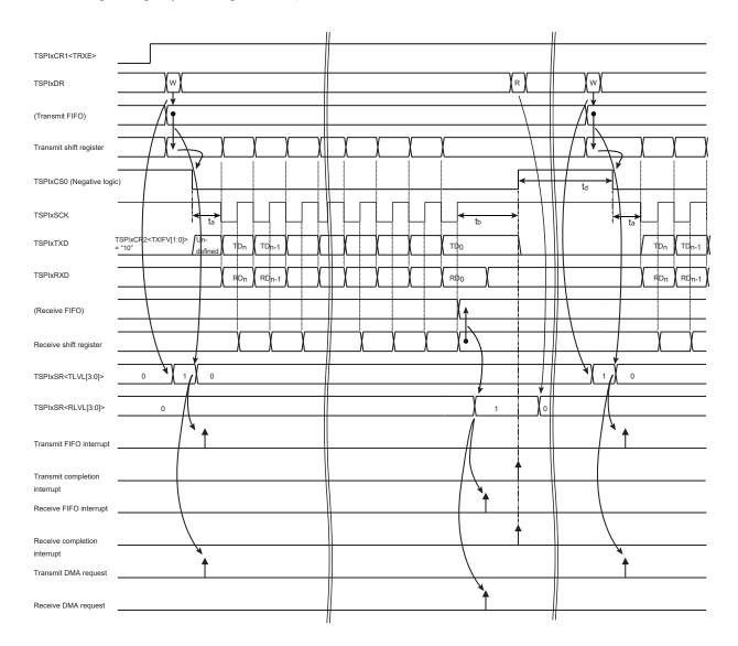
Figure 15-18 Operation example of full duplex communication
