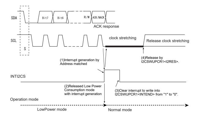
Figure 14-25 Address match Wake-up Function
