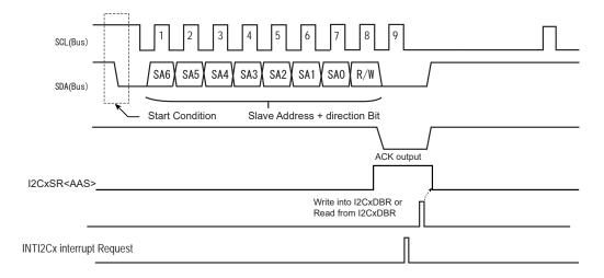
Figure 14-13 Slave address Match Detection Monitor
