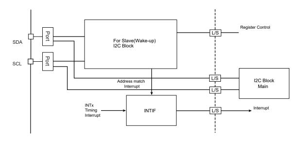
Figure 14-23 Wake-up Function Block
