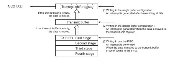
Figure 13-14 Transmit Buffer / FIFO Configuration Diagram
