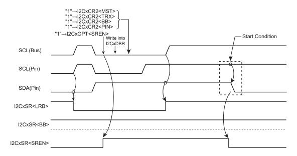
Figure 14-22 Timing Chart of Generating a Repeated Start
