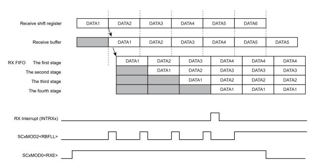
Figure 13-6 Receive FIFO Operation
