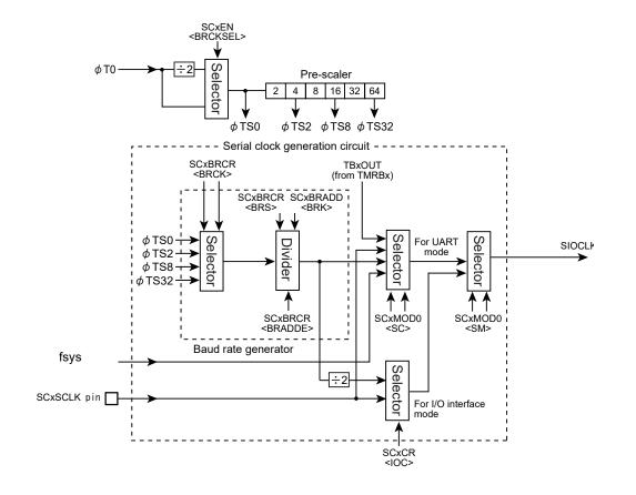
Figure 13-2 Serial clock generation circuit block diagram
