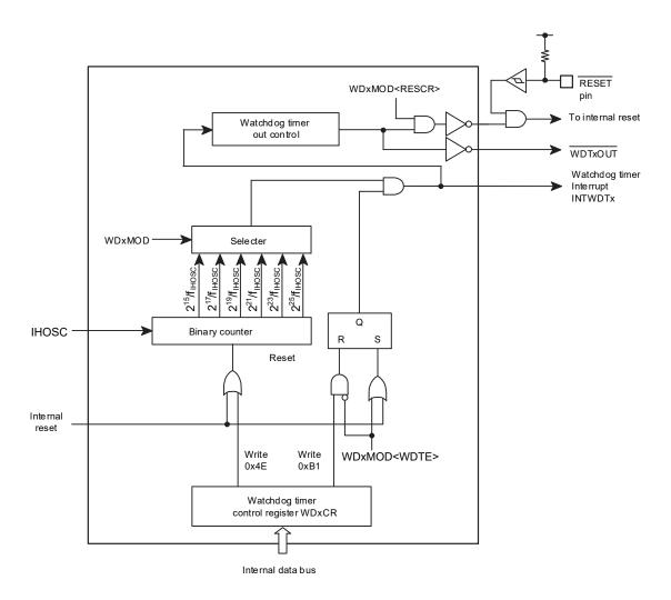
Figure 19-1 Block Diagram of the watchdog Timer
