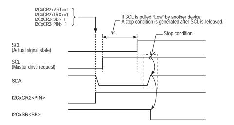
Figure 14-21 Generating the Stop Condition
