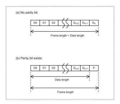
Figure 15-2 Data format schematic
