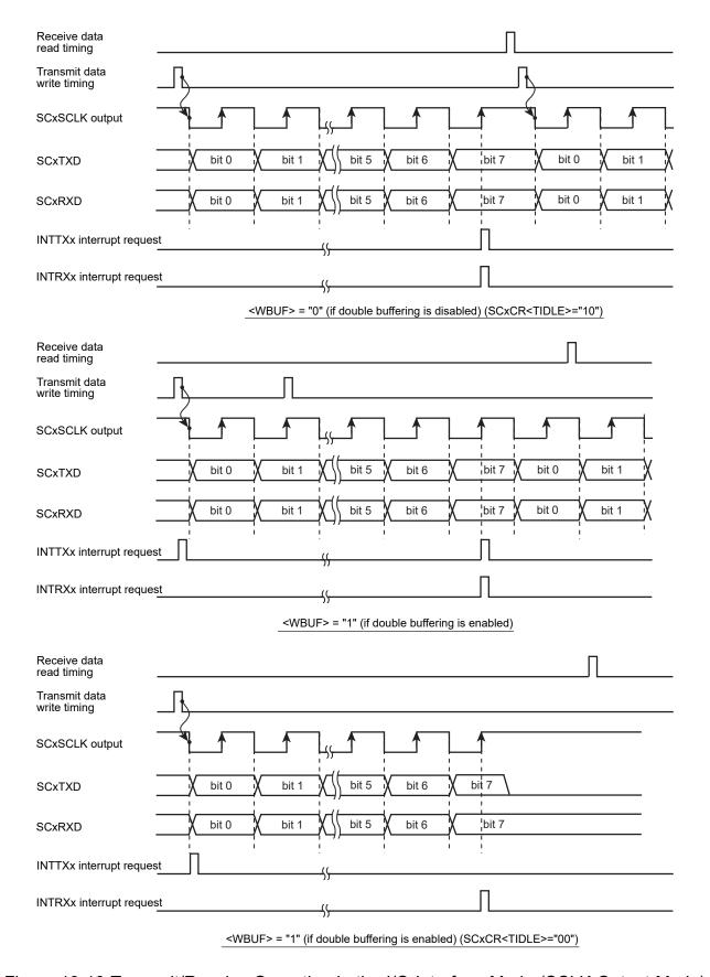
Figure 13-19 Transmit/Receive Operation in the I/O Interface Mode (SCLK Output Mode)
