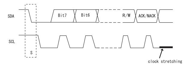
Figure 14-24 Clock stretch Function
