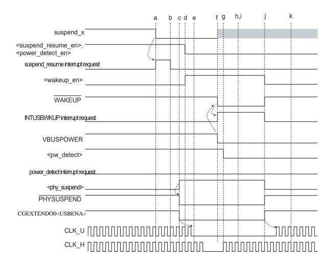
Figure 16-19 Operation of suspend/disconnect signals (to stop CLK H)
