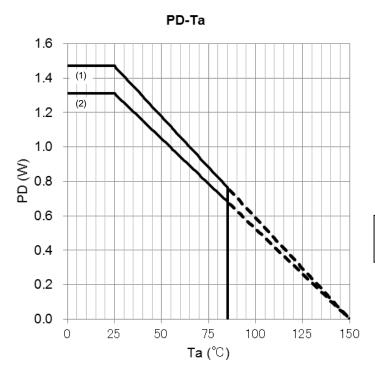
(1)PG type alone (2)When mounted on FWG type (75 × 114 × 1.6 mm, Cu area 20%, single-side glass epoxy)
