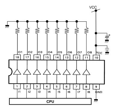
For voltage stabilization and noise rejection, please connect a stacked ceramic capacitor (0.01  $\mu$ F to 1 $\mu$ F) or an electrolytic capacitor (10  $\mu$ F to 100  $\mu$ F) to VCC line. The capacitor is recommended to be connected as close to the IC as possible.
