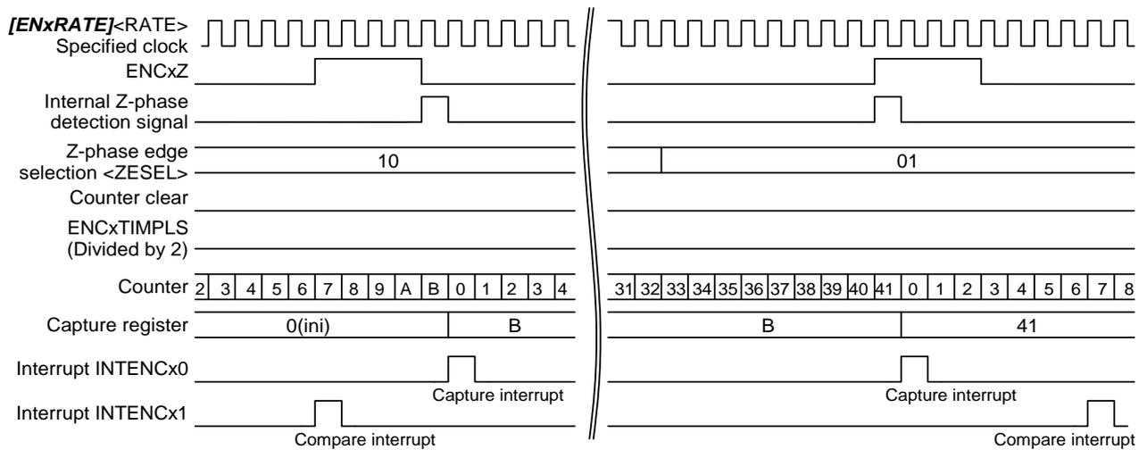
Figure 3.11 ENCxZ input is enabled ( $[ENxTNCR]<ZEN>=1$ )
