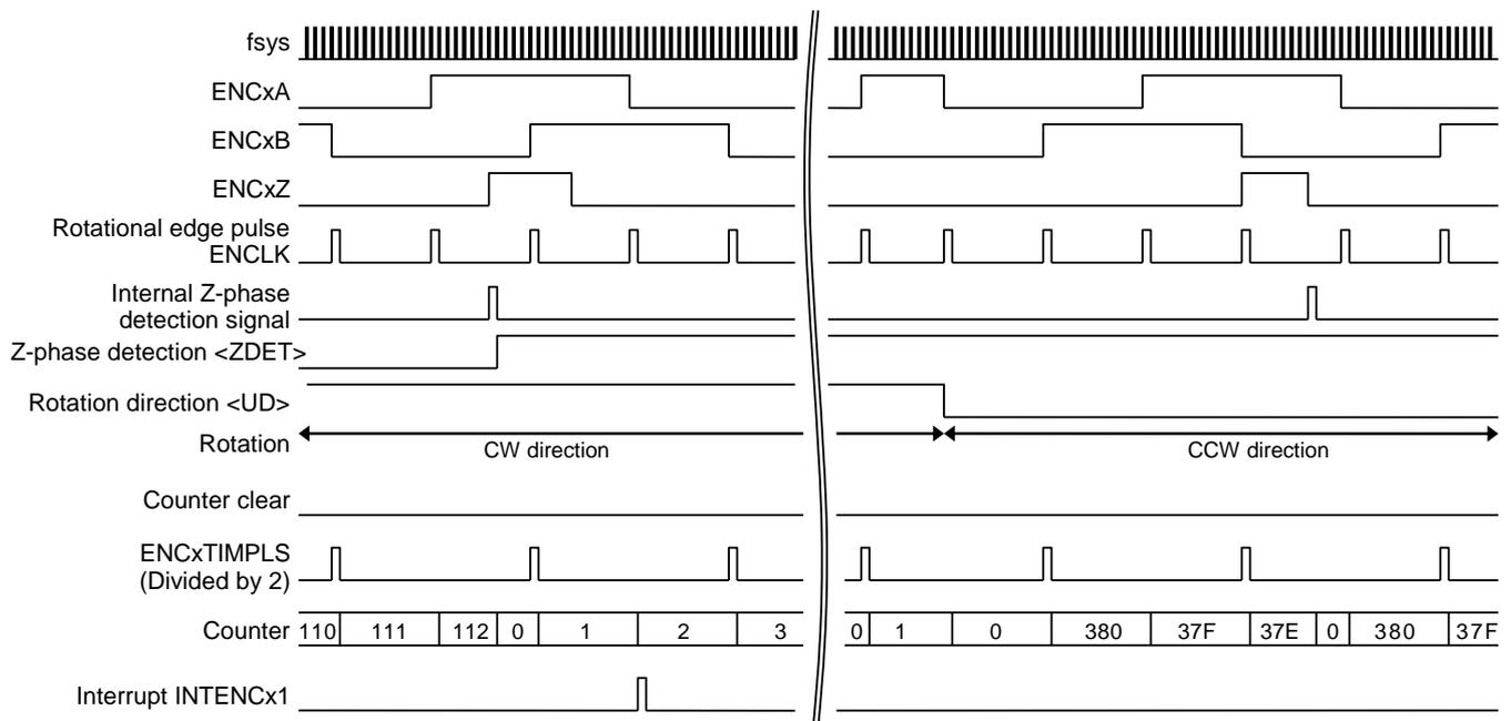
Figure 3.1 ENCxZ input enabled ( $[ENxTNCR]<ZEN>=1$ )
