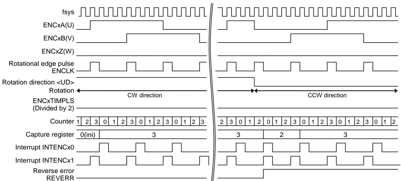
Figure 3.6 2-phase decoding ( $[ENxTNCR] \langle P3EN \rangle = 0$ )
