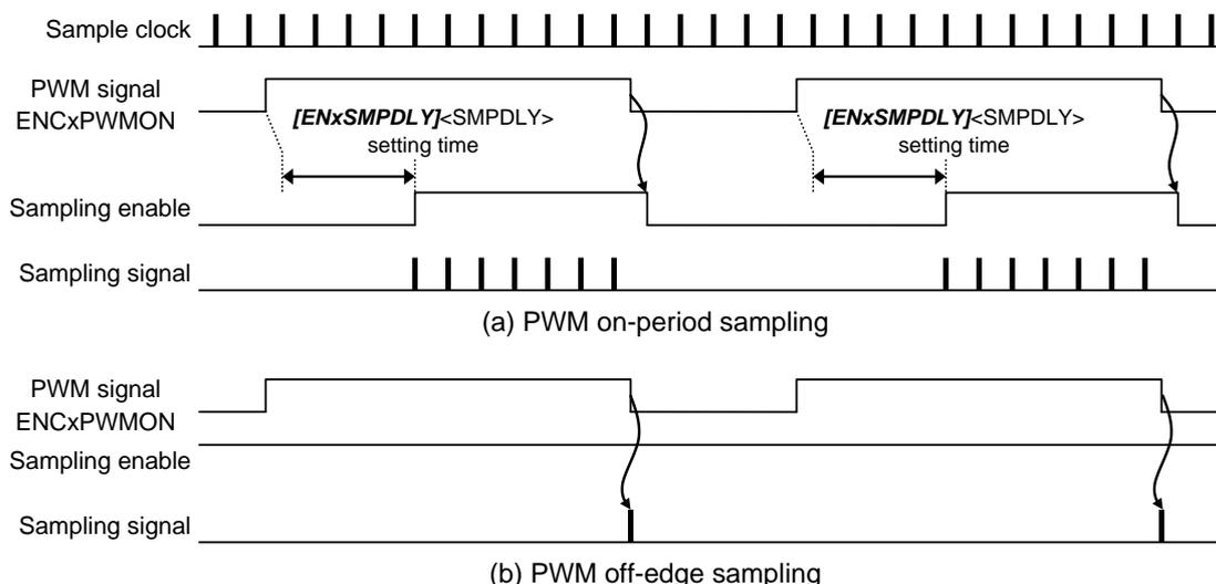
Figure 3.15 PWM synchronous sampling
