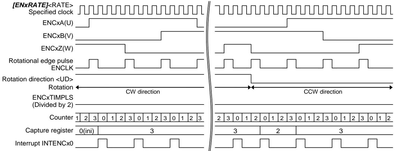
Figure 3.7 3-phase decoding ( $[ENxTNCR] <P3EN>=1$ )
