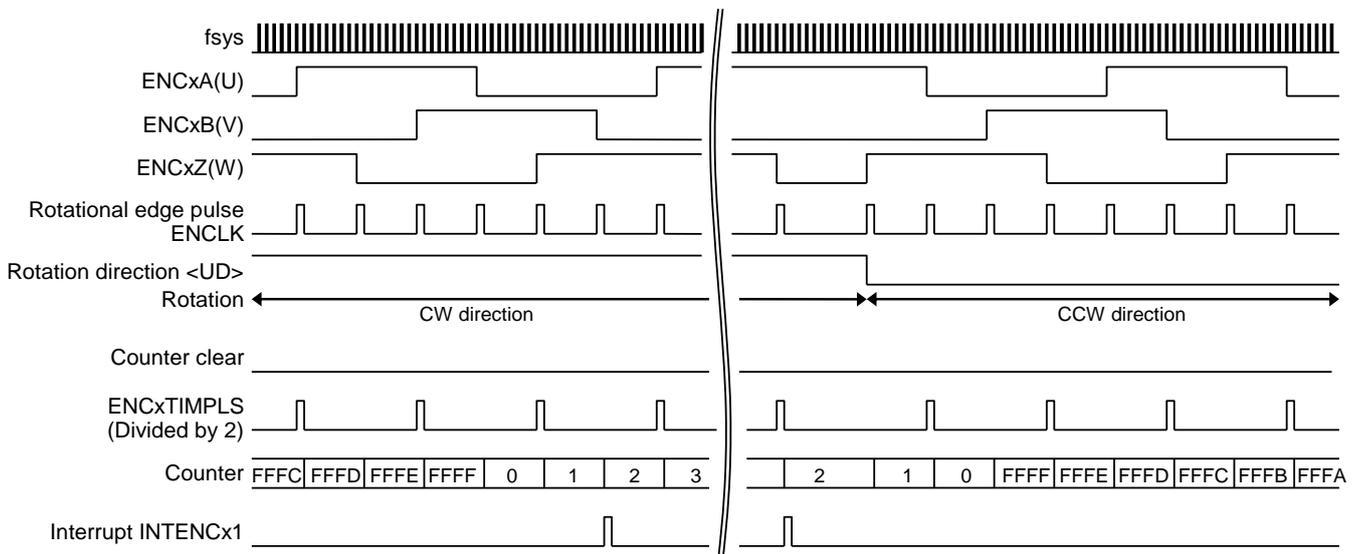
Figure 3.3 3-phase decoding ( $[ENxTNCR] < P3EN > = 1$ )
