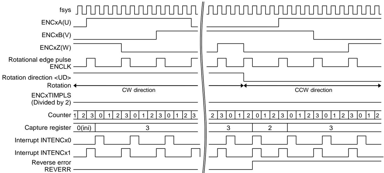
Figure 3.5 3-phase decoding ( $[ENxTNCR] \langle P3EN \rangle = 1$ )
