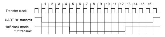
Figure 3.11 Data 0 transmission in the half clock mode
