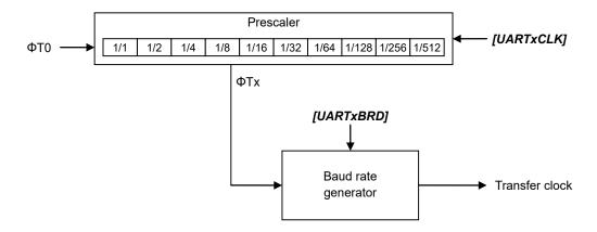
Figure 3.1 Transfer clock generator
