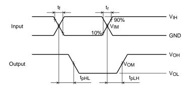
Figure 2  $t_{pLH}$ ,  $t_{pHL}$
