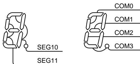
Figure 15-5 Example of COM, SEG Pin Connection (1/4 duty)
