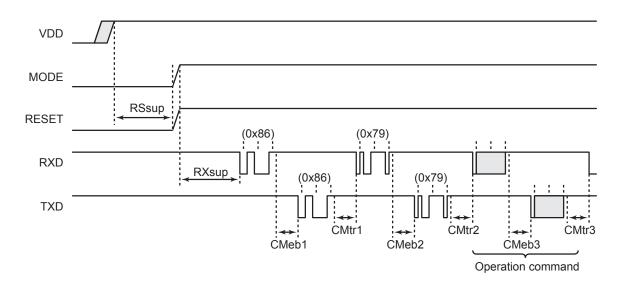
Figure 26-6 Reset Timing
