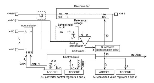
Figure 22-1 10-bit AD Converter
