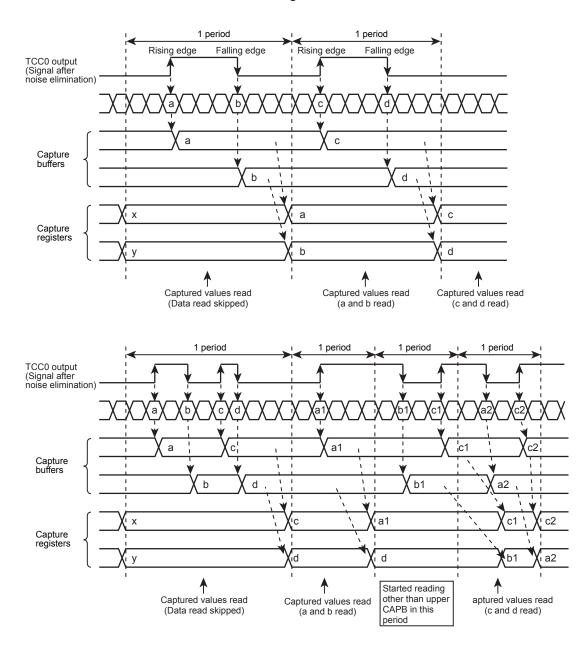
Figure 15-10 Example Operation in Trigger Capture Mode
