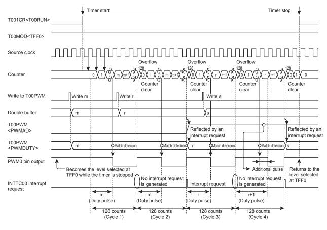
When the double buffer is enabled (T00MOD<DBE0>="1")
