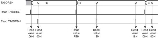
Figure 13-3 Timer Mode Timing Chart (Auto Capture)
