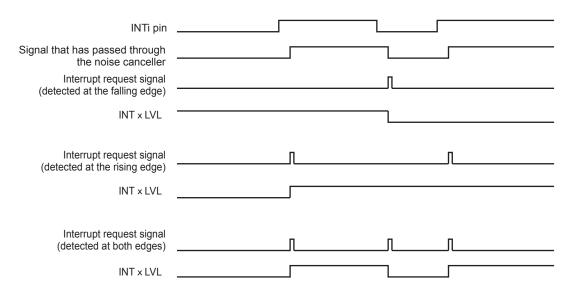
Note: The contents of EINTCRx<INTxLVL> are updated each time an interrupt request signal is generated.
