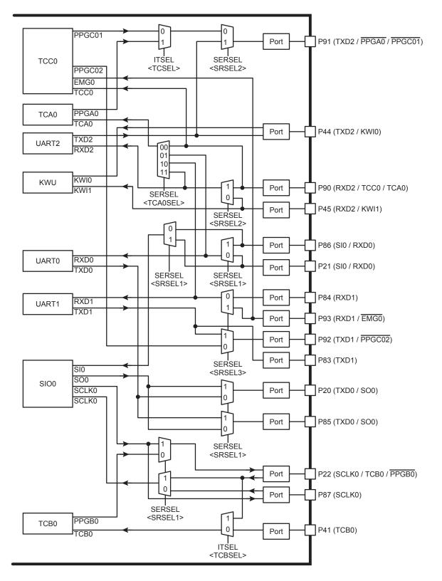
Figure 8-17 Peripheral function input/output select
