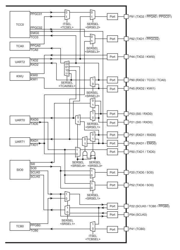
Figure 8-19 Peripheral function input/output select
