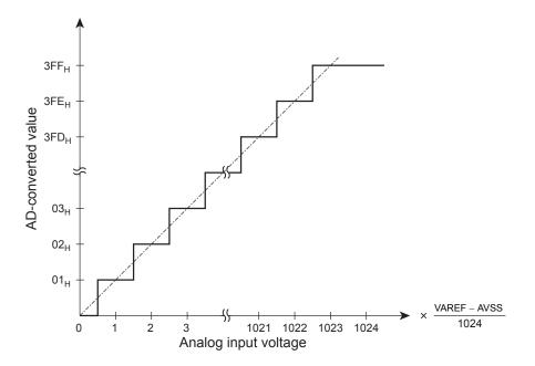
Figure 22-4 Relationships between Analog Input Voltages and AD-converted Values (typical values)
