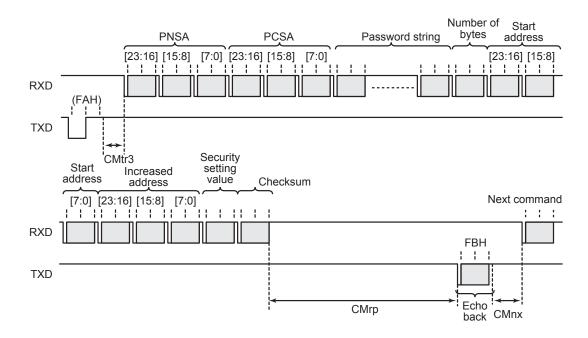
Figure 26-14 Flash Memory Security Setting Command
