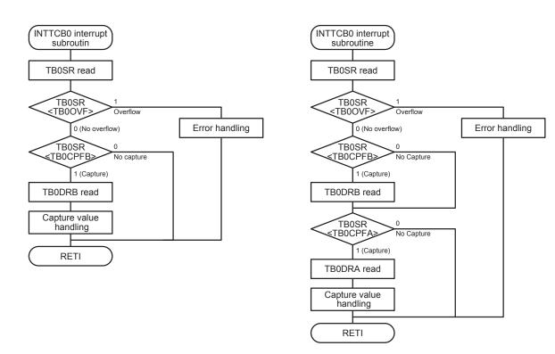
Interrupt process for single-edge capture
