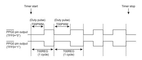
Figure 16-8 PPG0 Pulse Output
