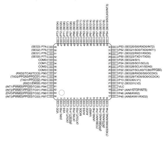
Figure 1-1 Pin Assignment (3/3)
