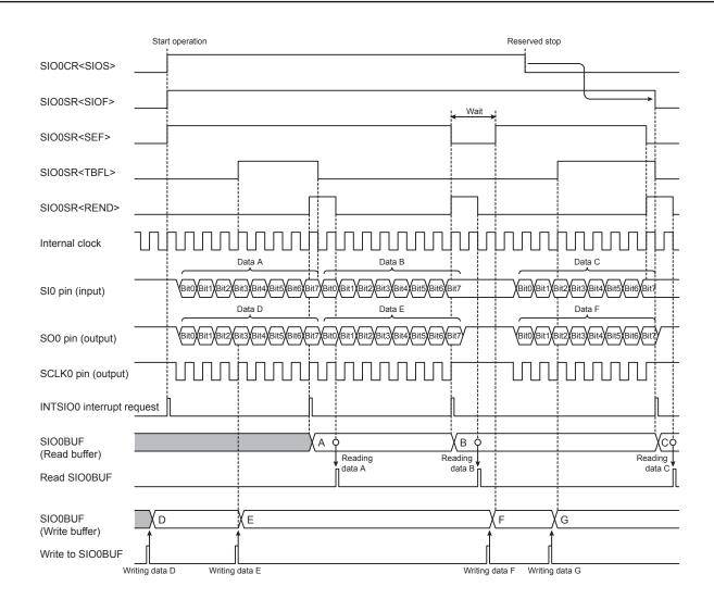
Figure 19-14 8-bit Transmit/Receive Mode (Internal Clock and Reserved Stop)
