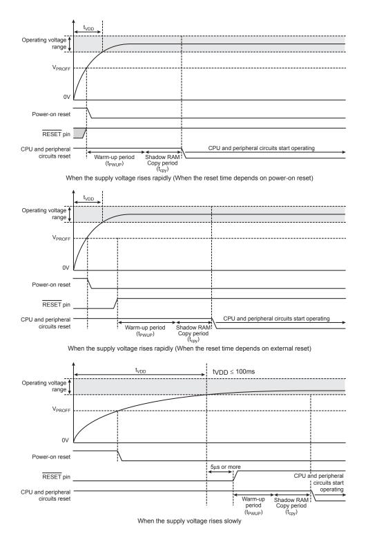
Figure 2-17 External Reset Input (During Power-Up)
