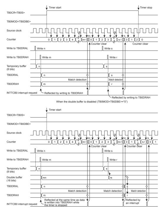
When the double buffer is enabled (TB0MOD<TB0DBE>="1")
