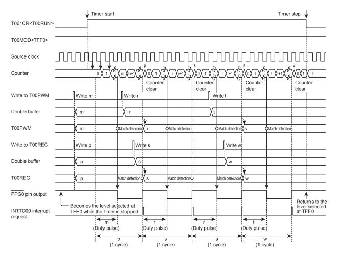
When the double buffer is enabled (T00MOD<DBE0>="1")
