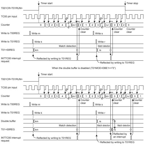
When the double buffer is enabled (T01MOD<DBE1>="1")
