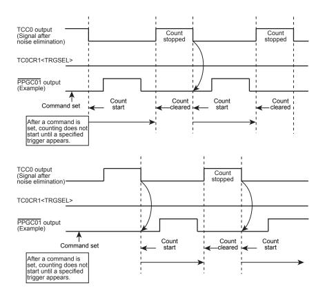
Figure 15-9 Example Operation in Trigger Start Mode
