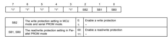
Note 1: Make sure to set "1" to the bit 7, 6, 5, 4 and 3 of the C register.
