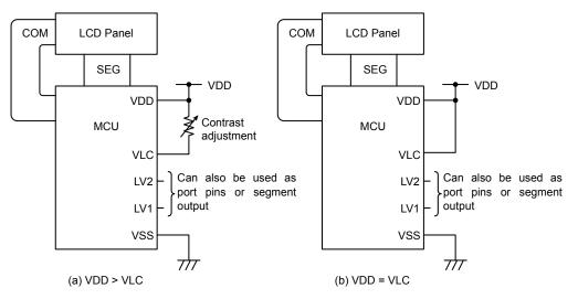
When internal bleeder resistance is used (LCDCR2<BRSEL>="1")
