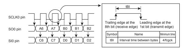
Figure 19-3 Interval time between bytes
