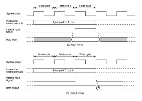
Figure 8-1 Input/Output Timing(Example)
