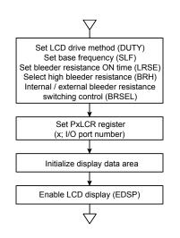
Figure 23-5 Flowchart for the LCD Driver Initialization
