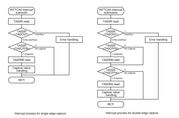
Figure 13-8 Example of capture process
