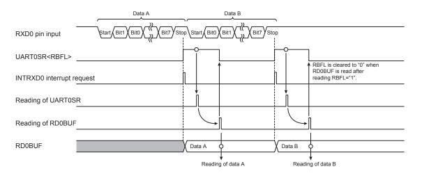
Figure 18-15 Occurrence of Receive Data Buffer Full
