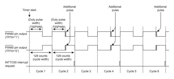
Figure 16-5 PWM0 Pulse Output
