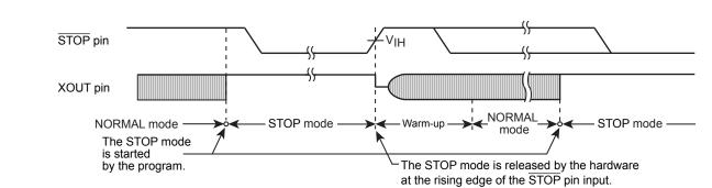
Note: If the rising edge is input to the STOP pin within 1 machine cycle after SYSCR1<STOP> is set to "1", the STOP mode will not be released.
