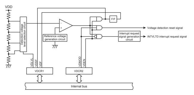
Figure 7-1 Voltage Detection Circuit
