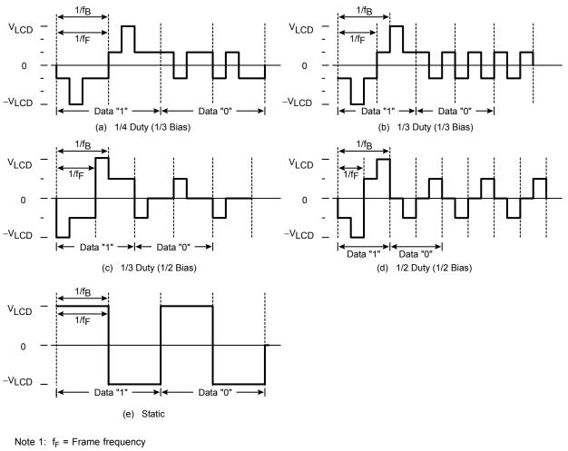
Note 2:  $f_B$  = Base frequency (LCDCR1<SLF>) Note 3:  $V_{LCD3}$  = LCD drive voltage ( =  $V_{LC} - V_{SS}$ )
