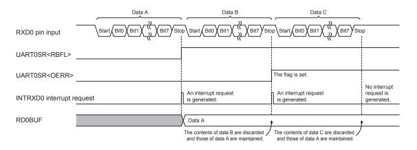
Figure 18-12 Generation of INTRXD0 Interrupt Request
