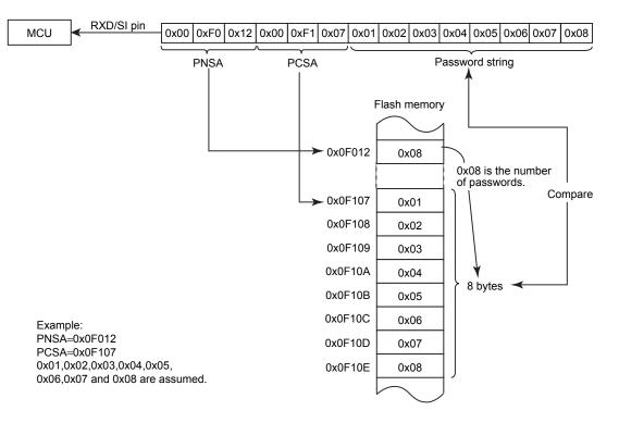
Figure 26-4 Example of How a Password Is Transmitted
