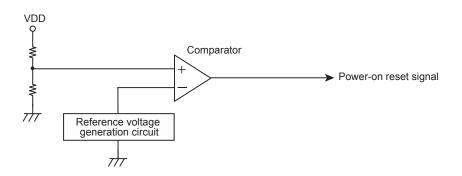
Figure 6-1 Power-on Reset Circuit
