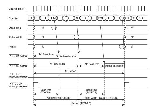
Figure 15-5 Example Operation in Variable Duty Mode: Command and Capture Start, Positive Logic, Continuous Output
