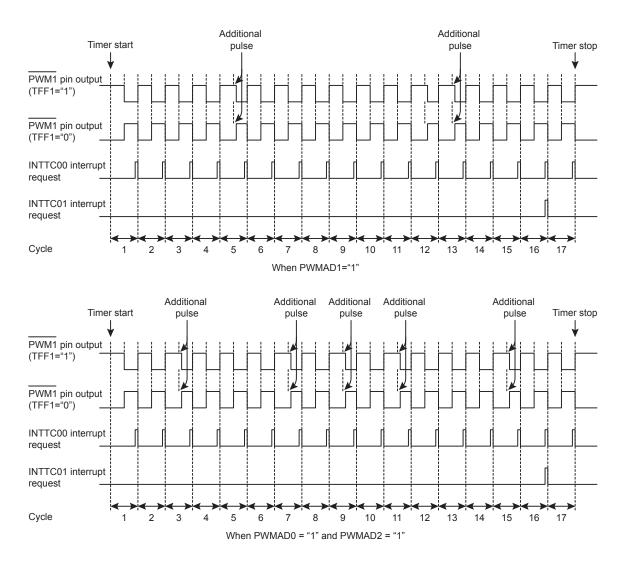
Figure 16-13 Examples of Inserting Additional Pulses
