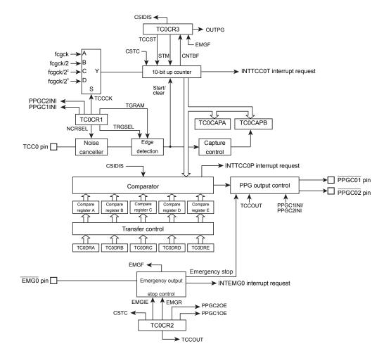
Figure 15-1 10-Bit Timer/Counter C0
