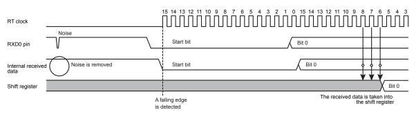
When the noise rejection circuit is used
