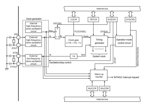
Figure 2-3 System Clock Controller
