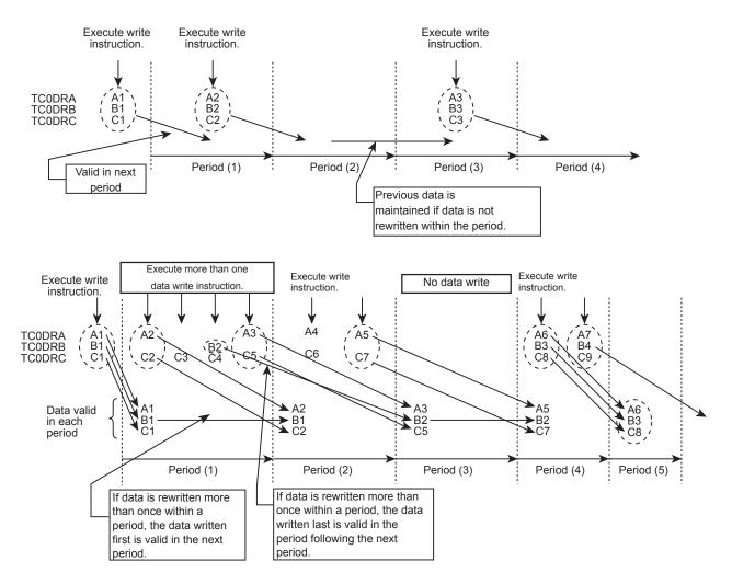
Figure 15-2 Example Configuration of Control/data Registers (1)
