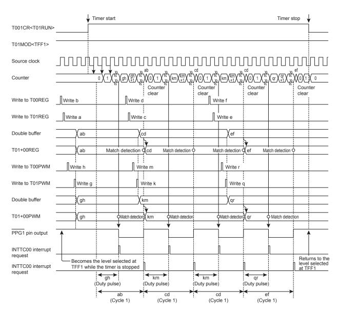
When the double buffer is enabled (T01MOD<DBE1>="1")
