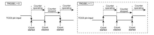
Figure 15-11 Trigger Input Signal
