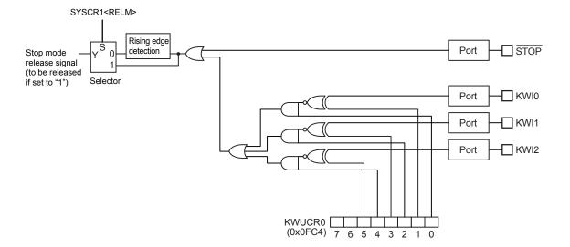
Figure 21-1 Key-on Wakeup Circuit
