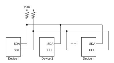
Figure 20-1 Device Connections
