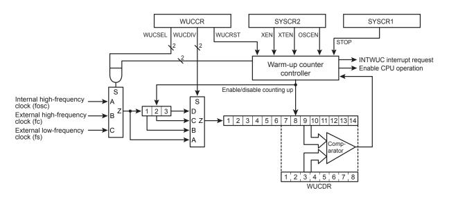
Figure 2-8 Warm-up Counter Circuit
