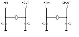
(1) High-frequency oscillation (2) Low-frequency oscillation
