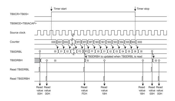
Figure 14-3 Timer Mode Timing Chart (Auto Capture)
