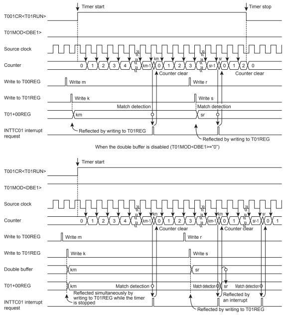
When the double buffer is enabled (T01MOD<DBE1>="1")
