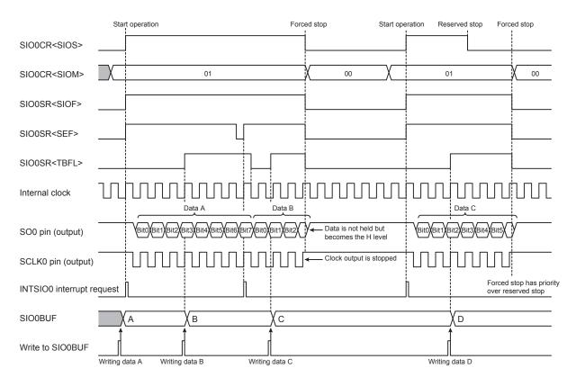
Figure 19-5 8-bit Transmit Mode (Internal Clock and Forced Stop)
