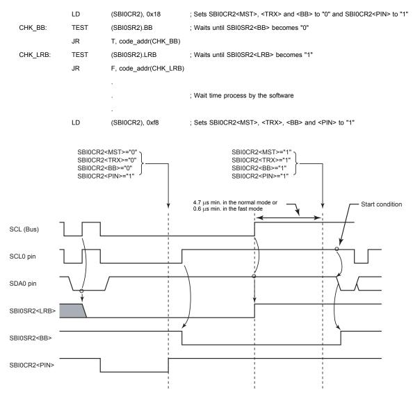
Figure 20-22 Timing Diagram When Restarting
