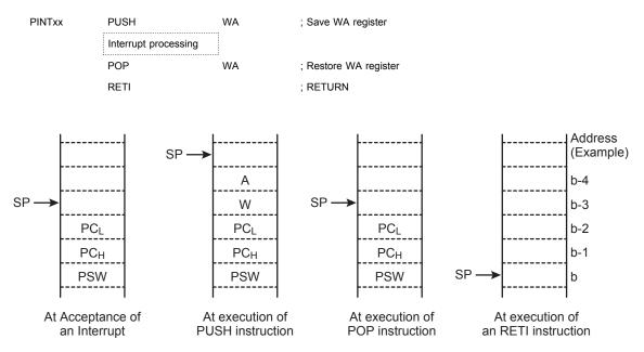
Figure 3-3 Saving/restoring general-purpose registers
