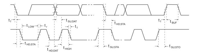
Figure 20-23 Definition of Timing (No. 1)
