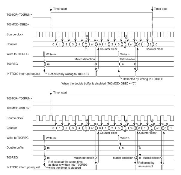
When the double buffer is enabled (T00MOD<DBE0>="1")
