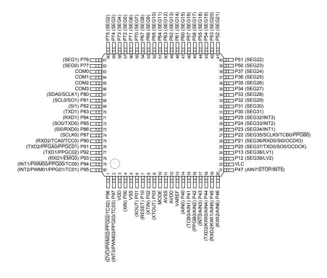
Figure 1-1 Pin Assignment (1/3)
