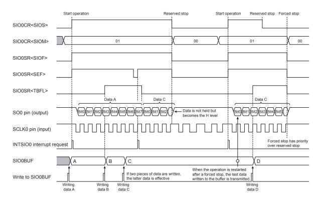
Figure 19-7 8-bit Transmit Mode (External Clock and Forced Stop)
