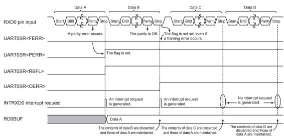
When a parity error occurs in the first received data and a framing error occurs in the second data
