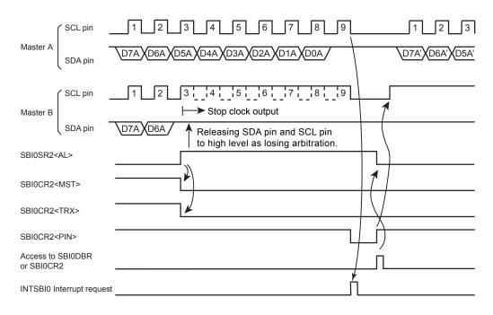
Figure 20-13 Example When Master B is a Serial Bus Interface Circuit
