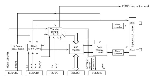
Figure 20-4 Serial Bus Interface 0 (SBI0)
