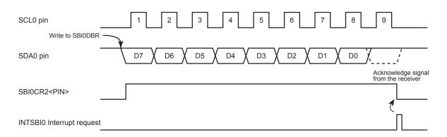
Figure 20-18 Example when SBI0CR1<BC>="000" and SBI0CR1<ACK>="1"
