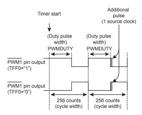
Figure 16-14 PWM1 Pin Output
