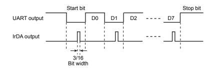
Figure 18-3 Example of Infrared Data Format (Comparison between Normal Output and Ir-DA Output)
