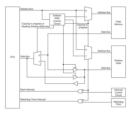
Figure 25-1 Configuration of the Shadow RAM Control Circuits
