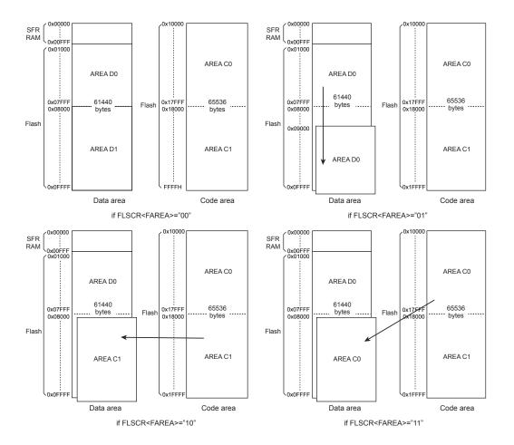
Figure 24-1 Area Switching Using the FLSCR1<FAREA> Setting
