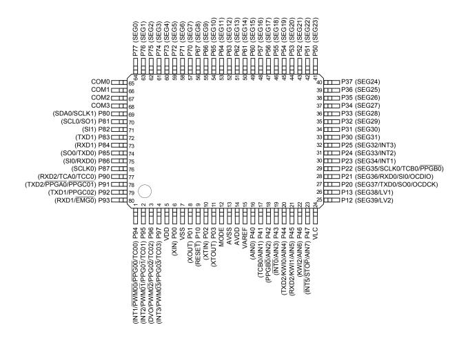
Figure 1-1 Pin Assignment (2/3)
