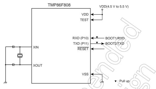
Figure 2.3.1 Serial PROM Mode Port Setting
