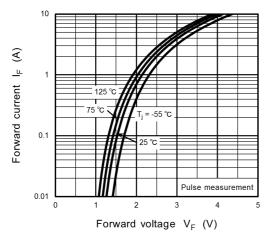
Fig. 10.1 I<sub>F</sub> - V<sub>F</sub> (Reference Maximum)
