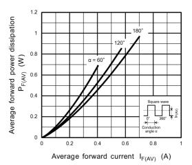
Fig. 10.2 P<sub>F(AV)</sub> - I<sub>F(AV)</sub>
