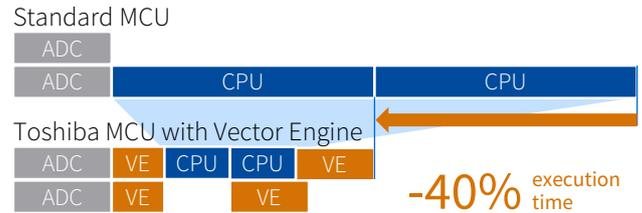
The **Vector Engine** significantly reduces CPU load and execution time for single and multi-axis motor control.
