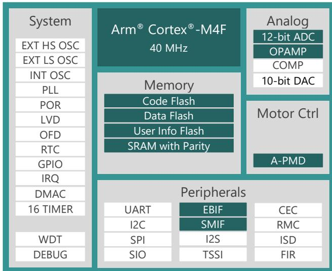
Besides a 12-bit ADC with up to 24 input channels and 1  $\mu$ s conversion time, the devices contain two units of 8-bit DAC and an Advanced Programmable Motor Driver (A-PMD) unit that can be used to perform general motor control or Power Factor Correction (PFC) operations.
