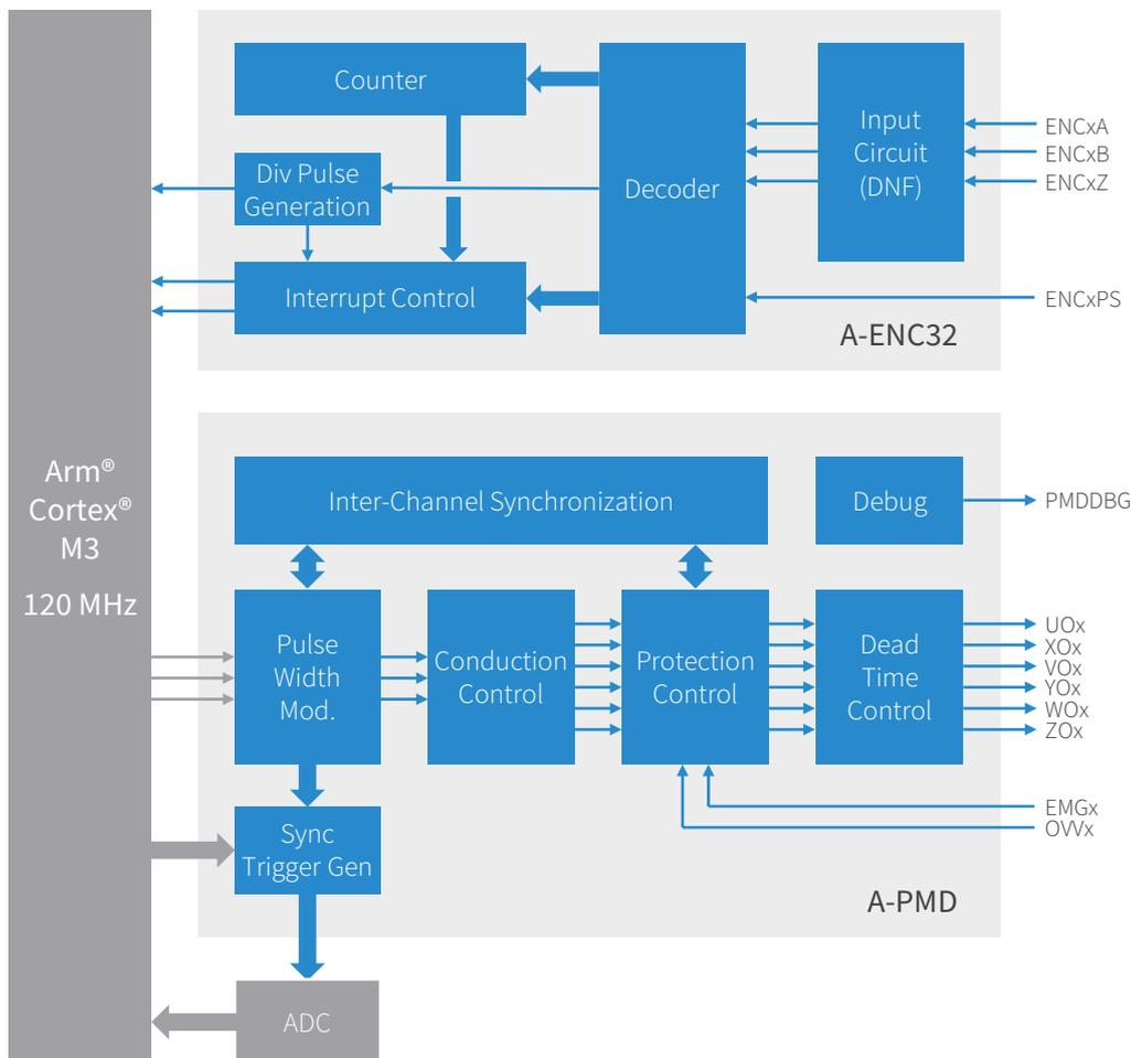
Toshiba’s [Advanced 32-bit Encoder Circuit \(A-ENC32\)](#) connects to external Hall sensors or incremental encoders.
