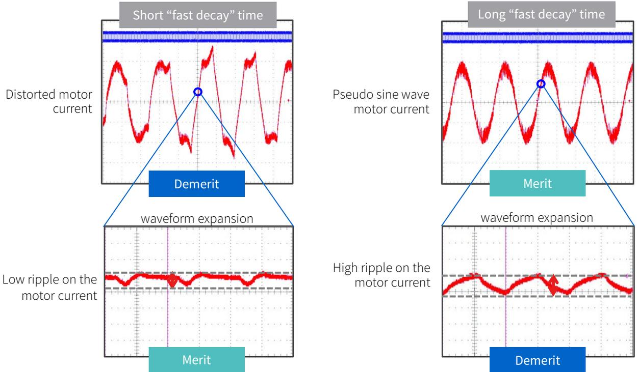
**Toshiba's Advanced Dynamic Mixed Decay (ADMD) technology** combines the best of both worlds and realizes pseudo sine wave motor control while reducing the ripple current. By this the maximum rotation speed can be increased without step loss (see picture below).
