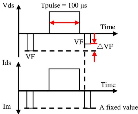
Fig. 7 In order to evaluate SOA, the change of forward-bias at drain when Ids is a fixed value is observed before and after power applying. The operating time (Tpulse) is 100 μs. The Ids is controlled by gate bias.
