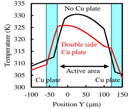
Fig. 8 The simulation results of temperature profile in the device with and without double side Cu film.
