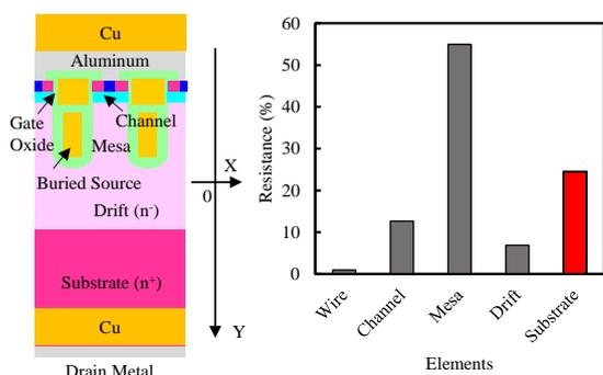
Fig. 5 The resistance ratio of some elements related to on-resistance (Ron) of vertical 40V Si power MOSFETs with buried source.
