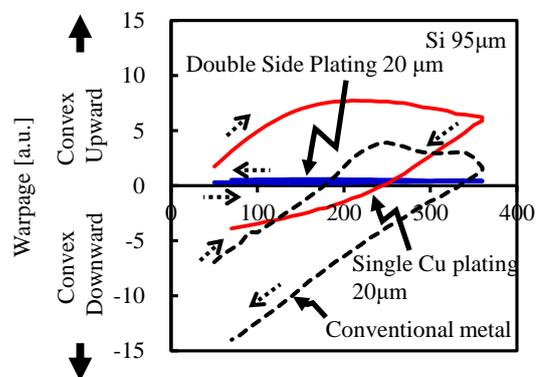
Fig. 4 Temperature dependence of warpage with single side and double side Cu plating.
