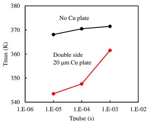
Fig. 10 The one pulse time dependence of the  $T_{MAX}$  for samples with and without double side 20  $\mu$ m Cu plate.
