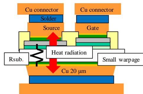
Fig. 1 The effect of vertical Si power MOSFETs with thin Si substrate and Cu double side plating.
