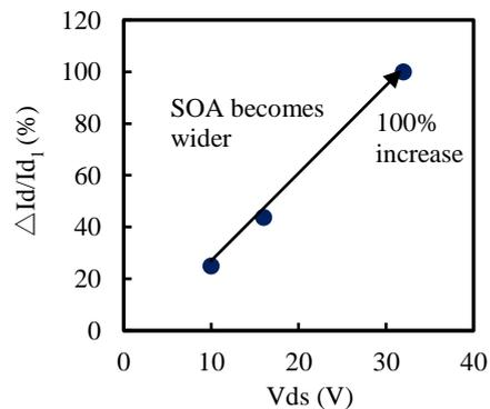
Fig. 9 The results of SOA with and without double side Cu film. The ratio of SOA ( $\Delta Id/Id_1$ ) becomes larger with increasing of Vds. 100 % larger SOA at Vds = 32V is observed thanks to 20μm Cu plate with larger heat capacity.
