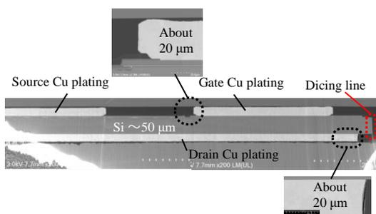
Fig. 3 The cross-sectional view of Si power MOS device with double side Cu plating. The thickness of both front and back is about 20 μm.
