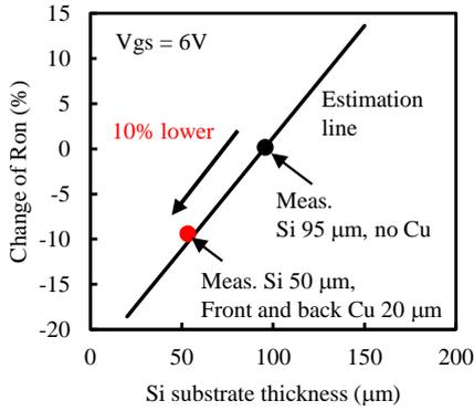
Fig. 6 The comparison of on-resistance between Si power MOSFETs with Si 95 μm and no Cu, and Si 50 μm and 20 μm Cu plate on both sides. The estimation line is calculated by the ratio as shown in Fig. 5.
