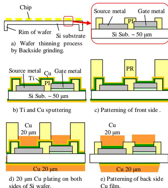
Fig. 2 Process flow of Cu double side plating for vertical Si power MOSFETs
