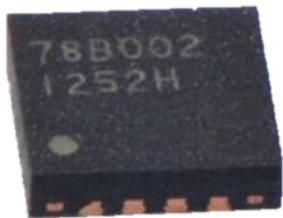
WQFN16 Package (3 mm x 3 mm x 0.75 mm)
