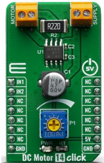
Figure 9: The H-bridge drivers can be quickly evaluated thanks to the DC Motor 14 Click board from MikroElektronika.
