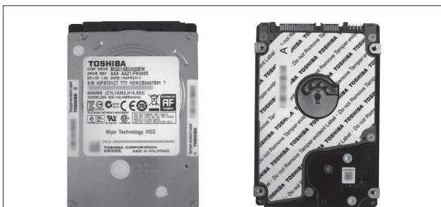
Fig. 3. Physical attack countermeasure using tamper seal — Example of a mobile HDD covered with tamper seal for protection against physical attacks
