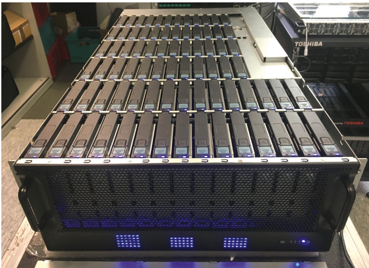
Picture 3: J4078-01 with 78 Toshiba HDDs
