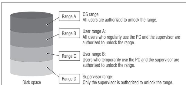
**Figure 2 Example of use of logical block address (LBA) ranges in disk space —**
