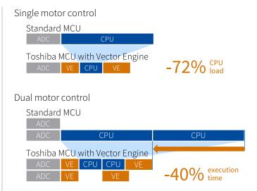
The Vector Engine significantly reduces CPU load and execution time for single and multi-axis motor control.
