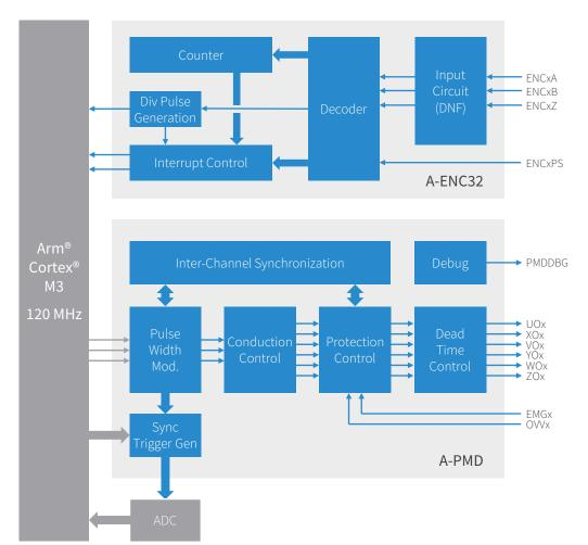
Toshiba's Advanced 32-bit Encoder Circuit (A-ENC32) connects to external Hall sensors or incremental encoders.
