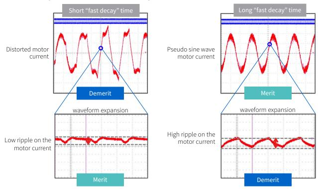
Toshiba's Advanced Dynamic Mixed Decay (ADMD) technology combines the best of both worlds and realizes pseudo sine wave motor control while reducing the ripple current. By this the maximum rotation speed can be increased without step loss (see picture below).
