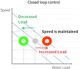
The device maintains constant rotation speed during load variation
