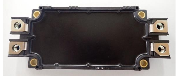
Fig. 3: 2200 V, 250A, 2in1 all SiC IMS module with an epoxy-potting encapsulation.
