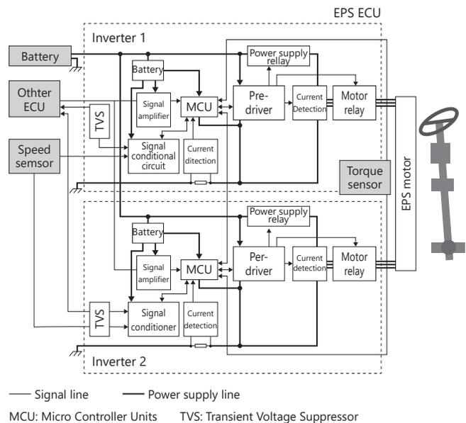
**Figure 2. Configuration of EPS system with redundancy**
