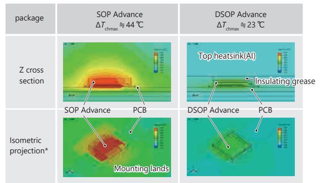
Applied power dissipation=2W, steady state
