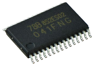
SSOP30 Package (10.2 mm x 7.6 mm x 1.6 mm)
