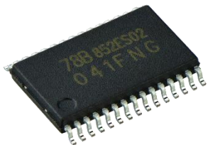
SSOP30-P-300-0.65 Package (10.2 x 7.6 x 1.6 mm)
