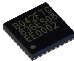
VQFN32 Package (5 x 5 x 1 mm)
