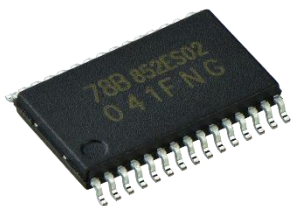
SSOP30-P-300-0.65 Package (10.2 x 7.6 x 1.6 mm)
