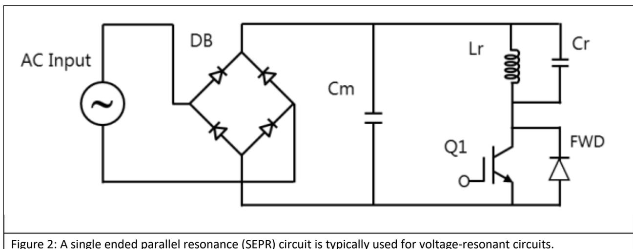
Figure 2: A single ended parallel resonance (SEPR) circuit is typically used for voltage-resonant circuits.
