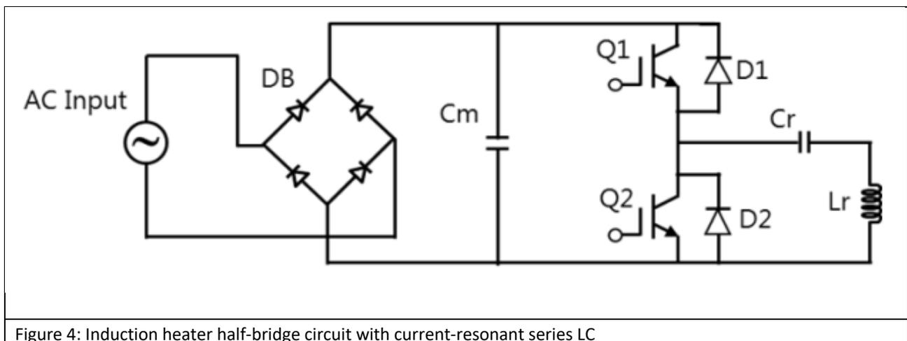
Figure 4: Induction heater half-bridge circuit with current-resonant series LC
