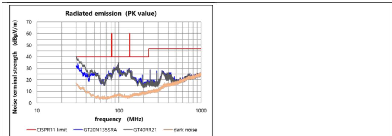
Figure 9: An improved turn-off results in 10dB more CISPR margin at 30 MHz for the same appliance
