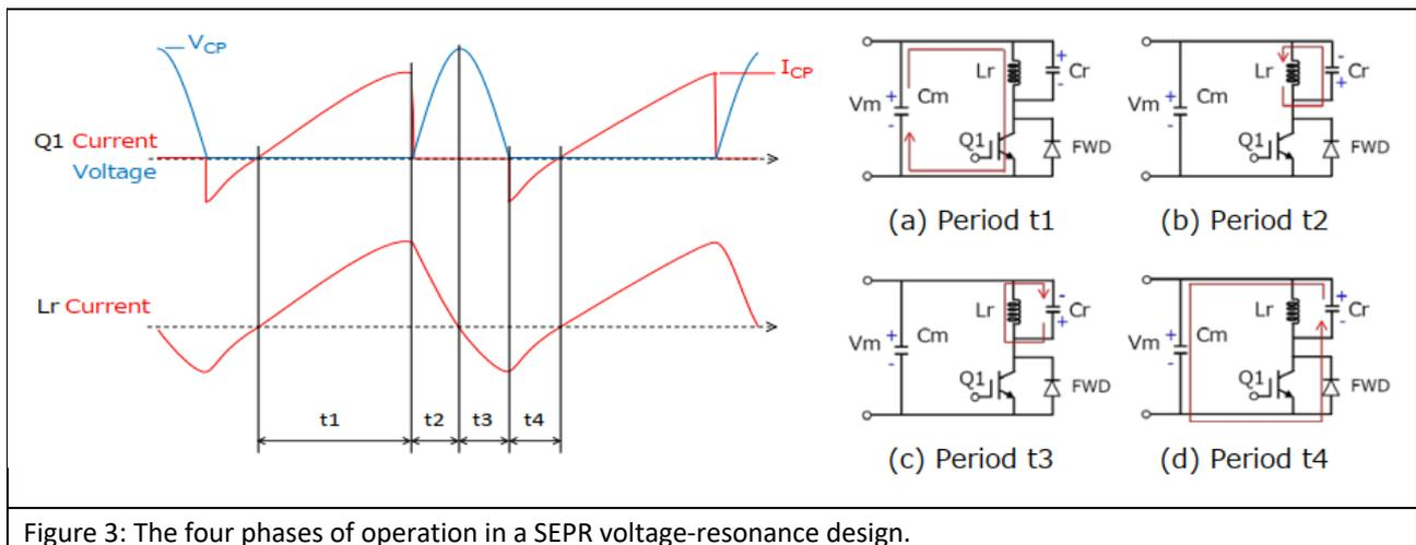
Figure 3: The four phases of operation in a SEPR voltage-resonance design.
