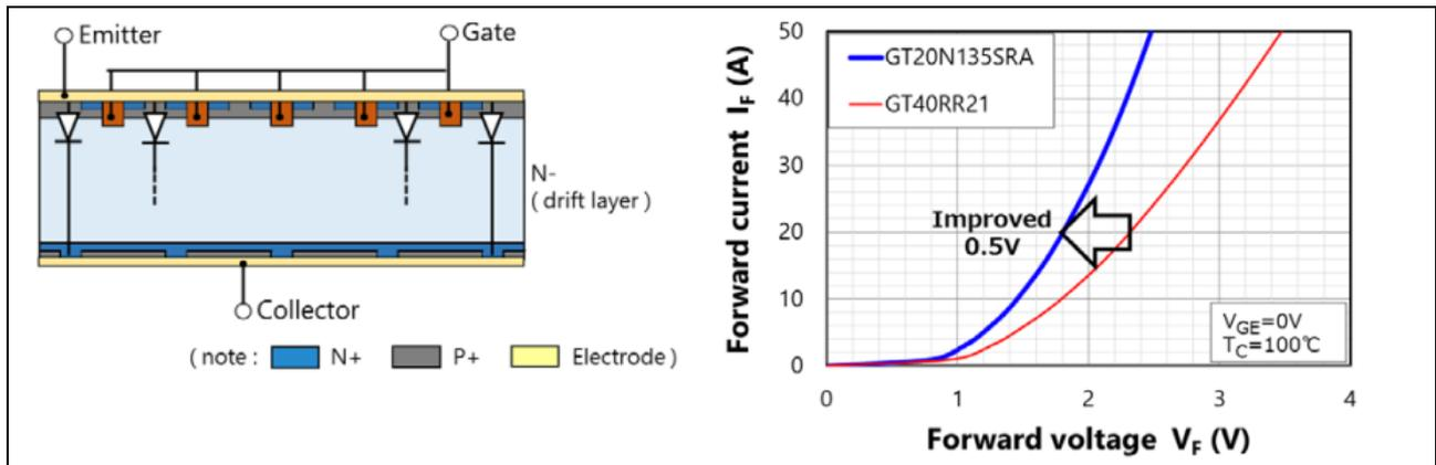
Figure 8: The body diode implementation of an RC-IGBT (left) and the improved  $V_F$  offered by the GT20N135SRA (right)
