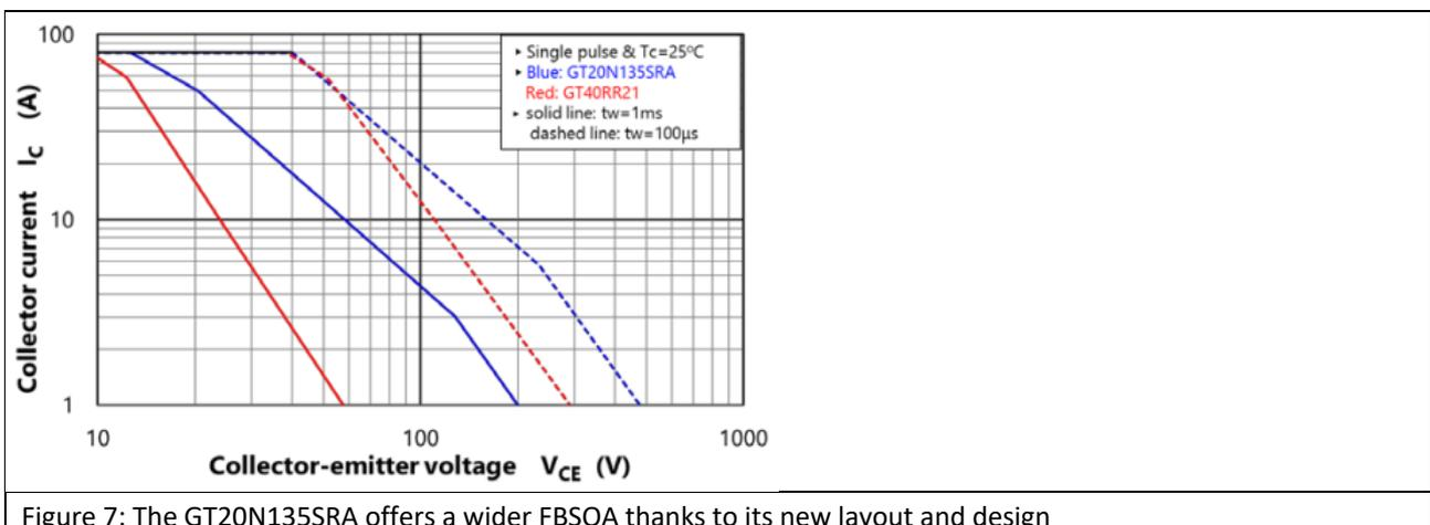
The wider FBSOA means that more current can flow in the IGBT but, due to losses, some of the energy flowing will need to be dissipated as heat. With a maximum  $R_{th(j-c)}$  of 0.48 °C/W, and assuming the IGBT needs to dissipate 35 W
