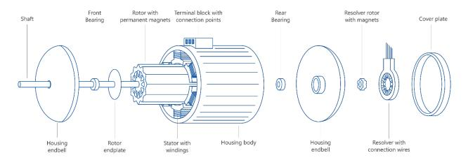
*Figure 1: An exploded view of the PMSM; the resolver adds to the cost, volume, and weight, while also adding another potential failure-point in the final system.*
