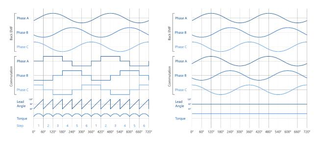
Figure 2: Torque ripple of a 6-step commutation (left) compared with FOC (right).
