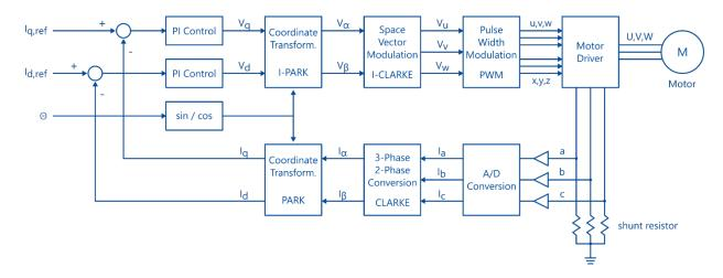
*Figure 3: FOC, or vector control, block diagram with transformations from the time variant threephase motor currents into the time invariant d, q reference frame.*
