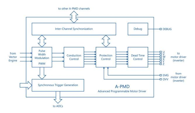
*Figure 8: Block diagram of the Advanced PMD, supporting the symmetrical PWM carriers required for the rotor estimation approach described.*
