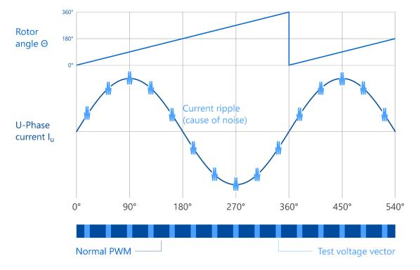
*Figure 5: The INFORM method applies intermittent high-frequency pulses to the phase control signal, but this can still result in higher-than-desired acoustic noise.*
