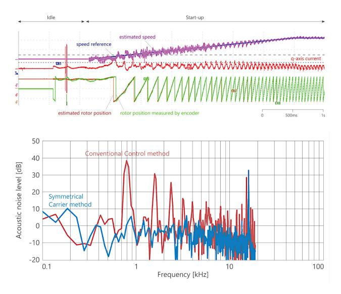
*Figure 7: A comparison of estimated and measured rotor position (using an encoder) (top) with a comparison of acoustic noise over frequency between symmetrical and conventional control methods.*
