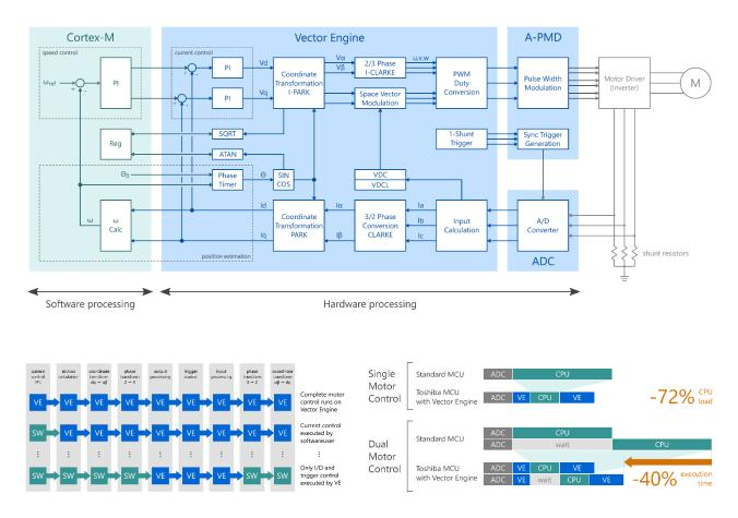
*Figure 9: The A-VE+ coprocessor can significantly offload the complexity of FOC PMSM algorithms, offers flexible configuration of the implementation, and can even support multi motor implementations.*
