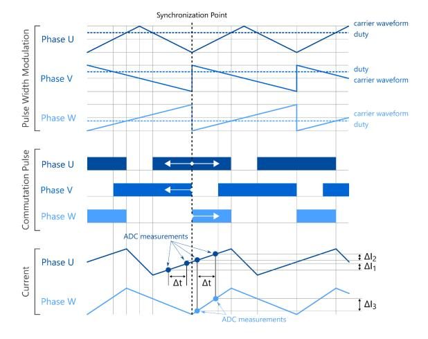
*Figure 6: Using three symmetric carriers the phase currents can be acquired when one of the three PWM outputs is inactive.*
