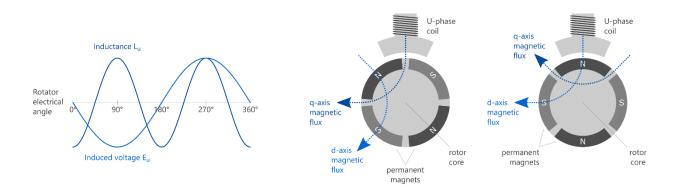
*Figure 4: The inductance of the stator coils varies at twice the rotor speed due to 'magnetic saliency' and can be used to determine rotor angle.*
