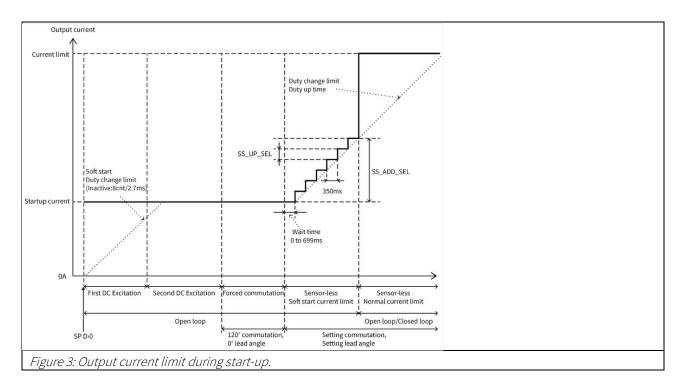
Once the motor rotates fast enough to generate a back-EMF usable for the control algorithm, the TC78B011FTG switches to sensorless control with the current limit set for normal operation. If selected, closed-loop speed control is also engaged.
