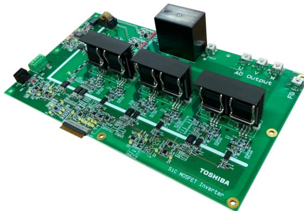
Figure 11: 400V motor inverter featuring four-pin TW045Z120C 3 rd generation SiC MOSFETs.
