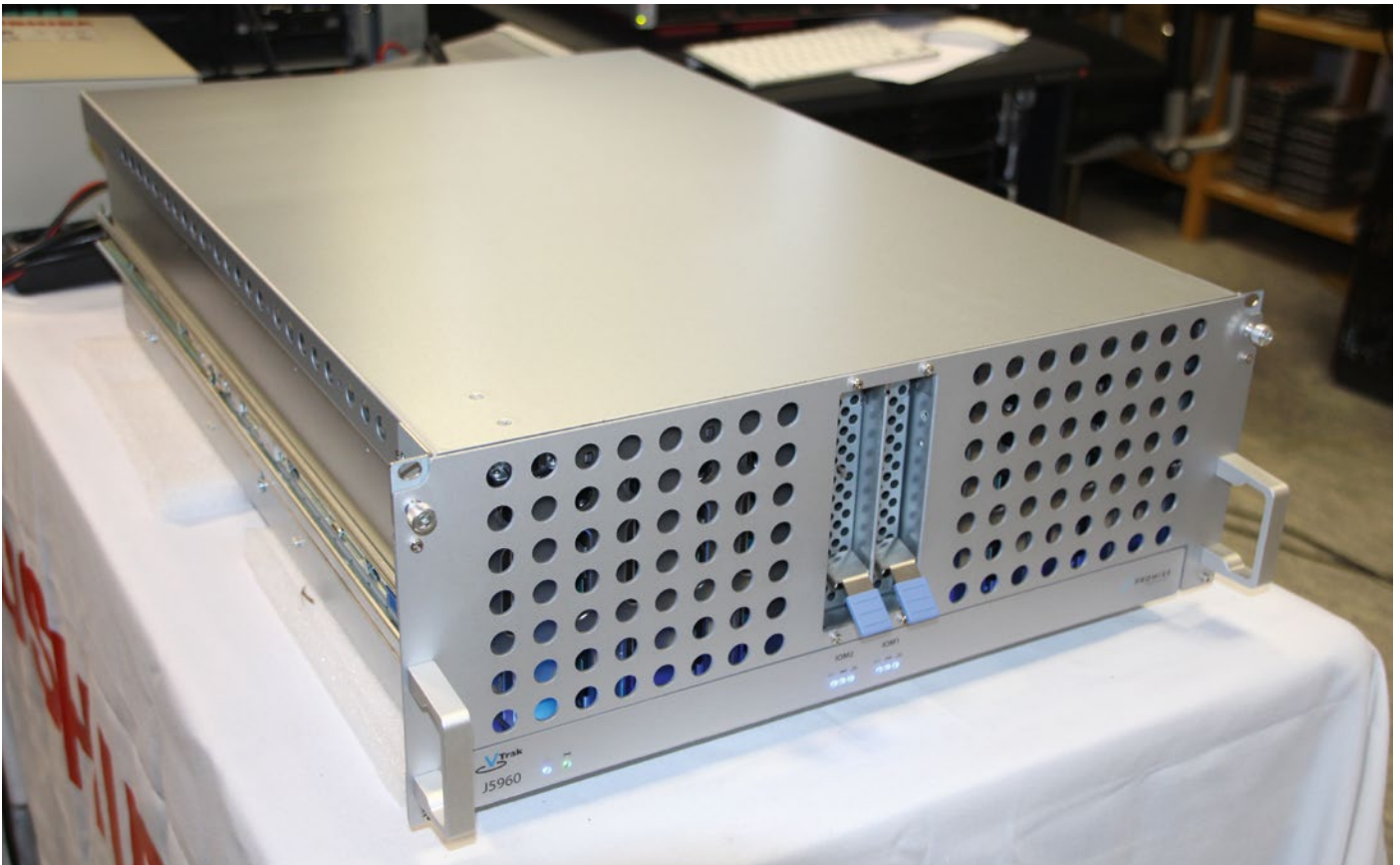
Picture 1: PROMISE VTrak J5960 JBOD in the Toshiba lab.
