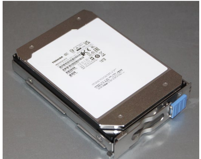
Picture 3: Toshiba HDD MG09SCA18TE in PROMISE tray.
