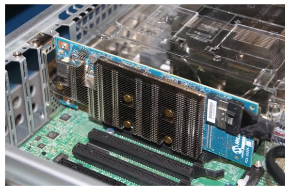
Picture 2: Microchip Adaptec® SmartRAID 3204-8i in server
