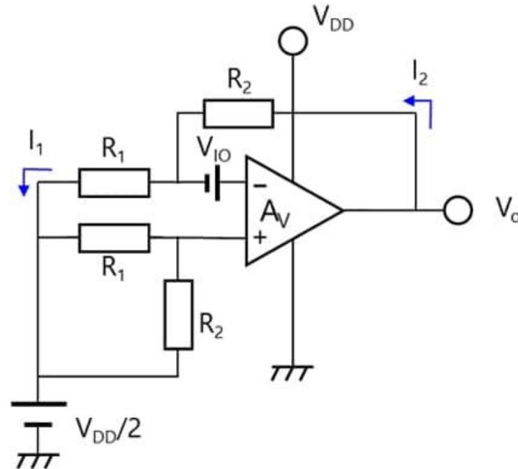
Test circuit for the input offset voltage
