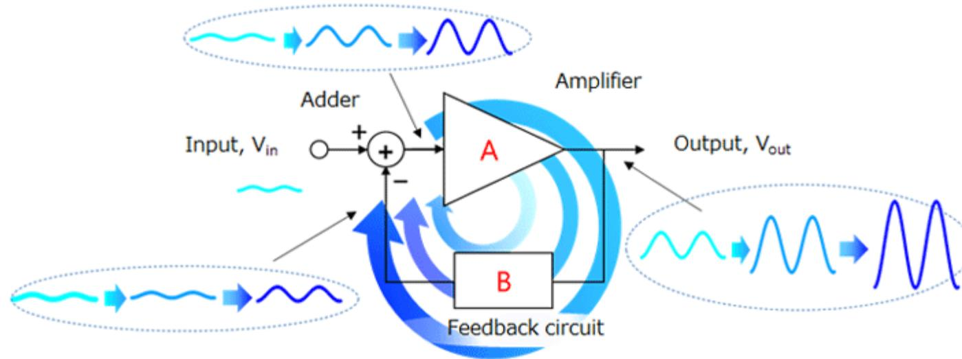
Growth of an unwanted signal through a feedback circuit
