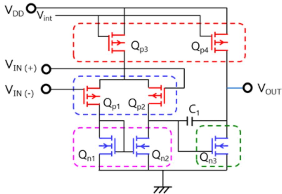
Simplified equivalent circuit for an op-amp
