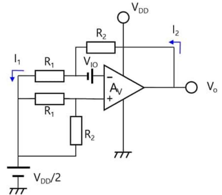
Test circuit for the input offset voltage
