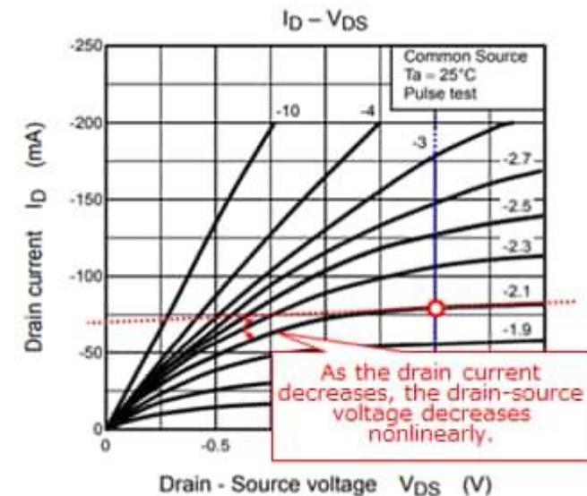
Example of  $I_D$ - $V_{DS}$  curves of a P-channel MOSFET
