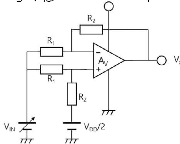
Test circuit for CMRR and CMV<sub>IN</sub>
