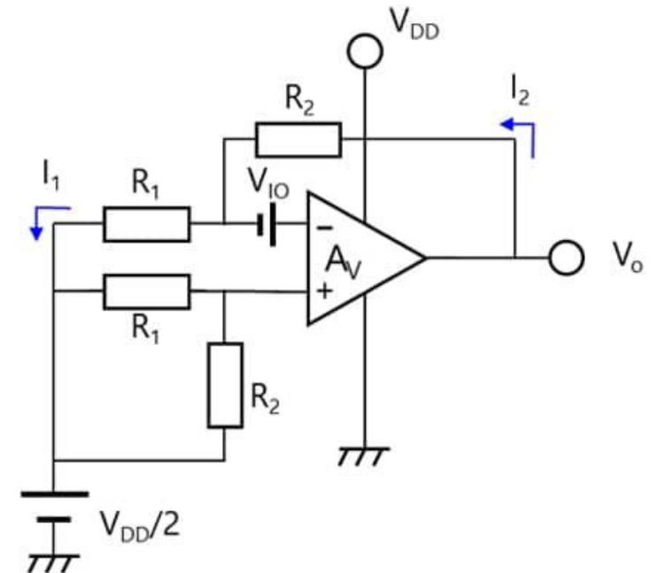
Test circuit for the input offset voltage
