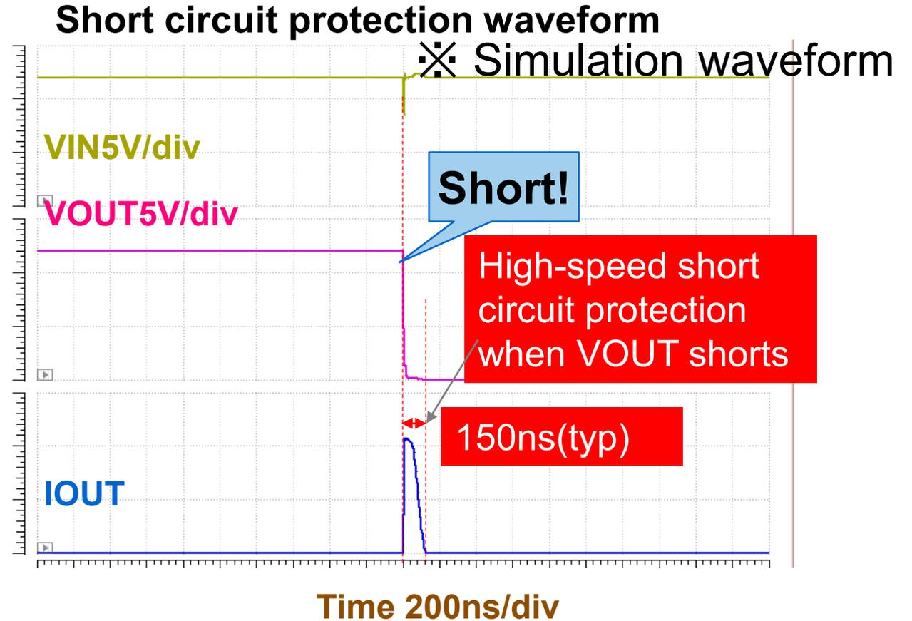
Because of the faster off-time, damage and destruction of the subsequent IC can be reduced
