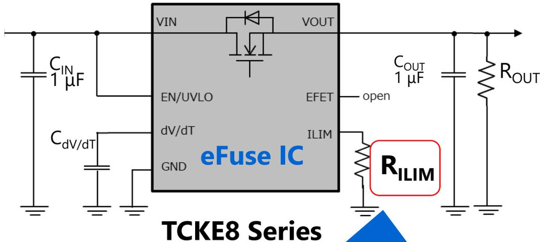
For the overcurrent limit with an external resistor ( $R_{ILIM}$ ) can be set to 0.5 ~ 5A
