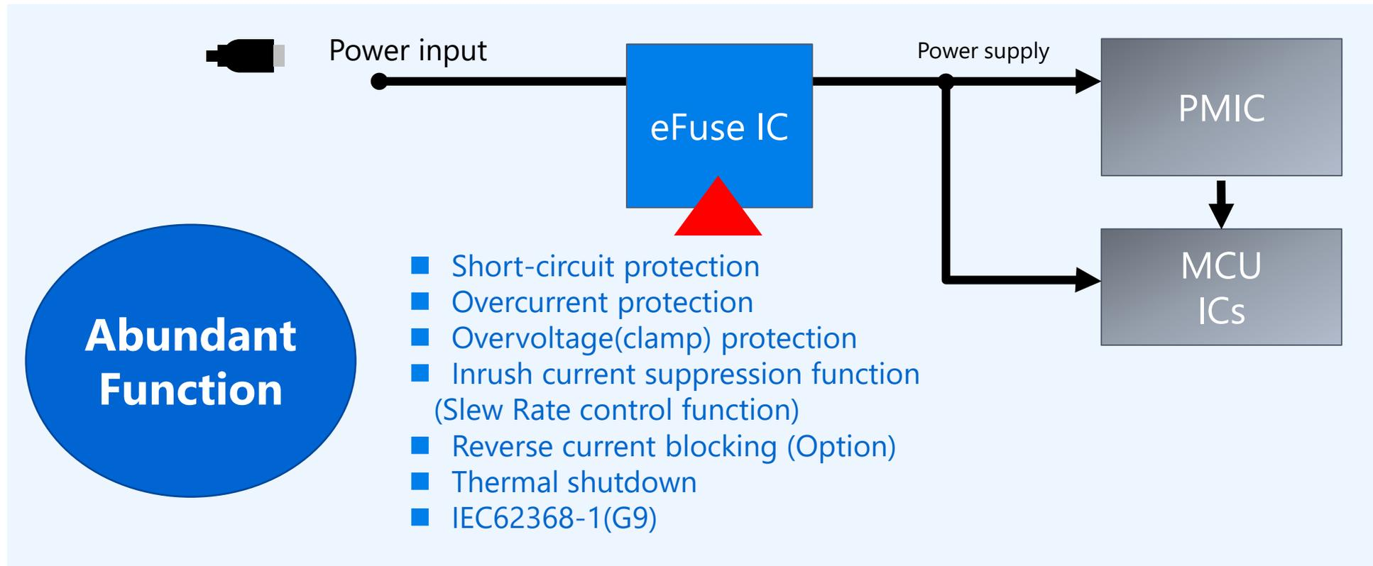
The eFuse IC has a high-performance, high-precision protection function built into one package, which is not found in conventional fuses.
