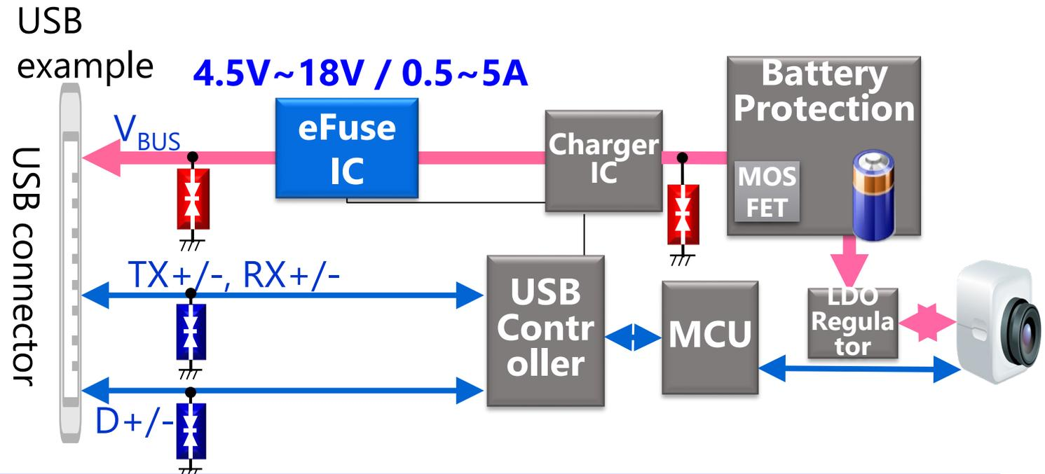
From Load SW and MOSFET to eFuse to comply with USB-terminal standards Switching is proceeding. It is important to use it in combination with ESD, etc.
