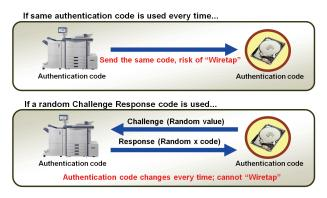
The Wipe2 SED is able to judge the authentication code from a Wipe2 enabled host by comparing the completing the pre-determined challenge and response protocol process inside the secure SED device.
