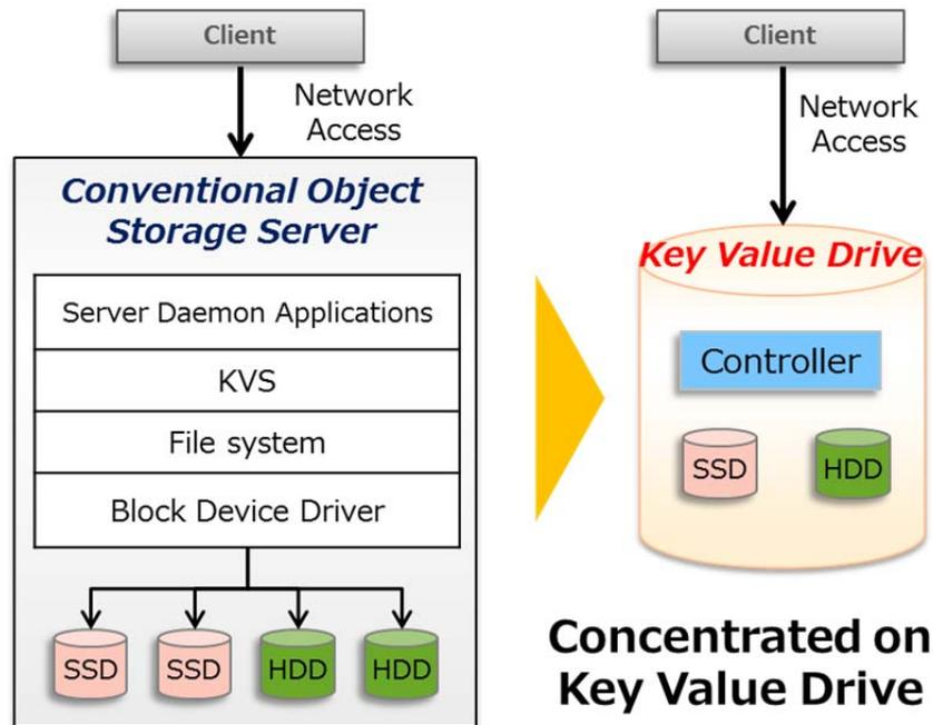
Figure 2 Server-Based Object Storage vs. Key Value Drive
