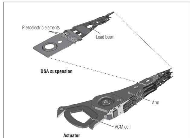
**Figure 7 Newly developed actuator with DSA suspension —**
