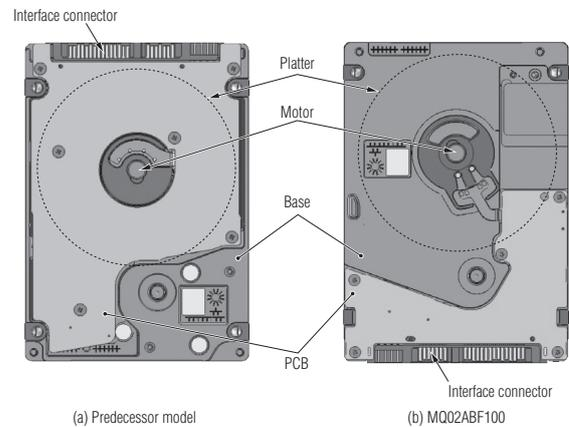
**Figure 4 Comparison of base shape of predecessor model and base shape optimized for MQ02ABF100 —**
