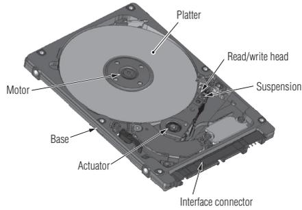
**Figure 1 Internal structure of MQ02ABF100 —**
