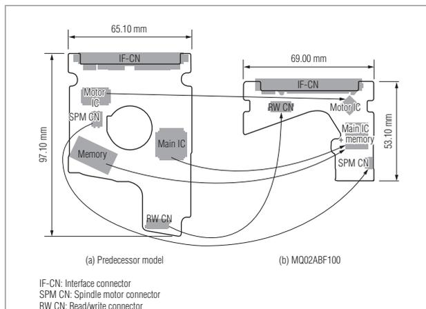
**Figure 6 Reduction of printed circuit board —**
