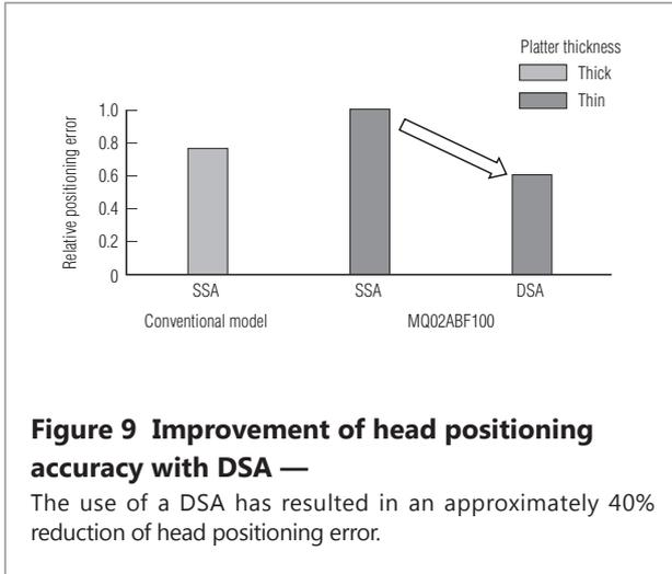
**Figure 9 Improvement of head positioning accuracy with DSA —**
