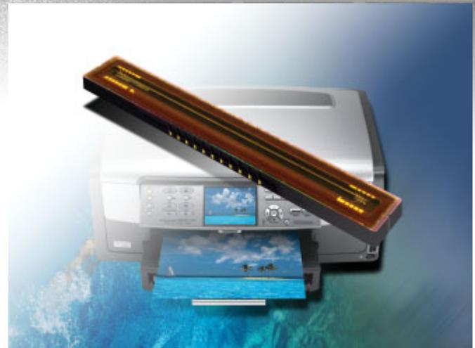
The TCD2914BFG is Toshiba's first CCD linear imaging product based on a single-layer CCD structure. It is a high sensitive and low dark current 10680 elements x 3-line CCD color image sensor with a 10680 elements x 1 line CCD B/W image sensor, a CCD drive circuit and a clamp circuit. Engineered for scanner applications, the device provides a 48-lines/mm 1200 dpi resolution across A4-size paper. It is operated by a 5.0 volt (V) pulse and 12V power supply.
