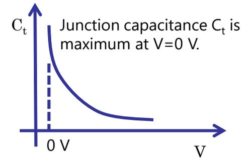
Fig. 2-10(b) Characteristic of junction capacitance of SBD
