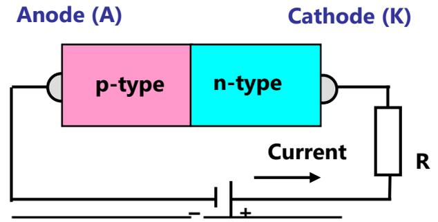
Fig. 2-4(a) Structure and connection of Zener diode
