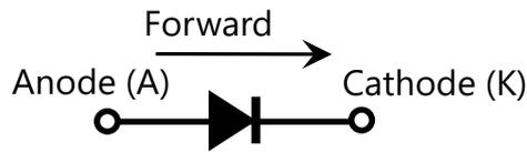
Fig. 2-1(a) Symbol of diode and names of its electrodes
