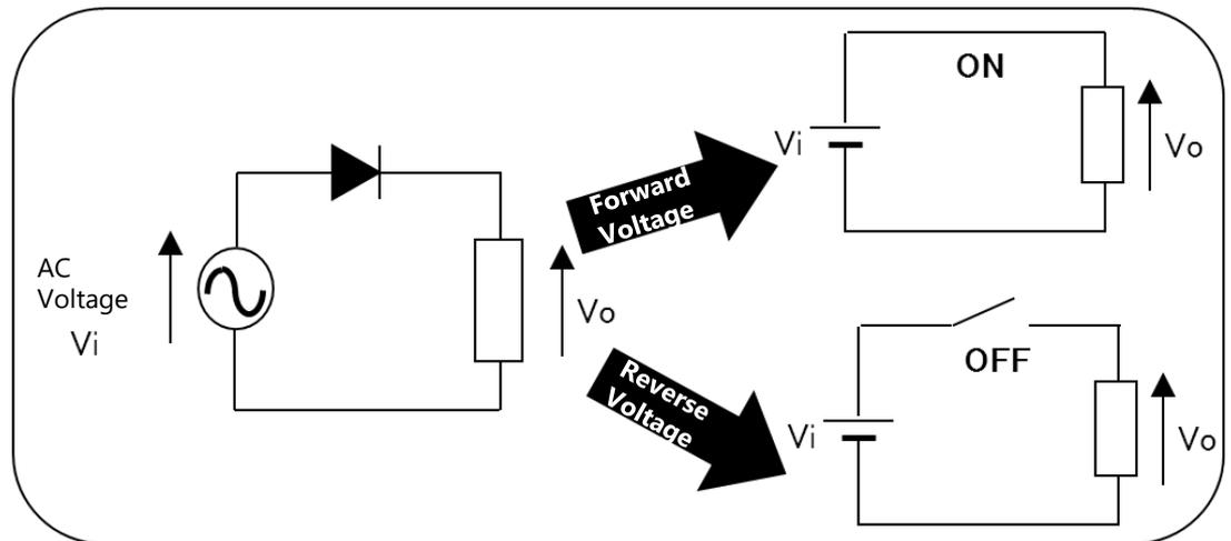
Fig. 2-2 Typical function of diode
