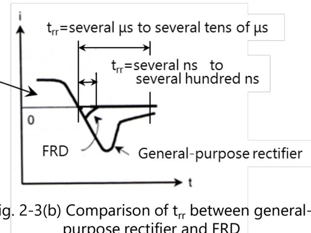
Fig. 2-3(b) Comparison of  $t_{rr}$  between general-purpose rectifier and FRD
