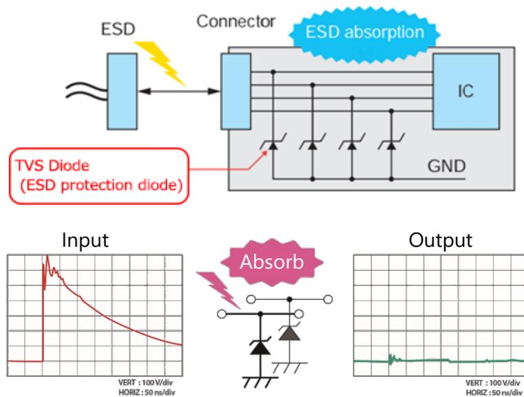
By using TVS diode (ESD protection diode), it can absorb intrusive ESD, prevent malfunction of the circuit, protect device such as IC !
