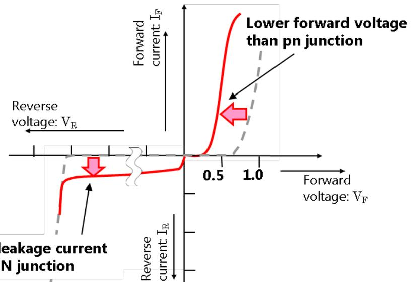
Fig. 2-9(b) Electrical characteristic of Schottky barrier diode
