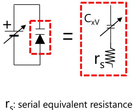
$r_s$ : serial equivalent resistance
