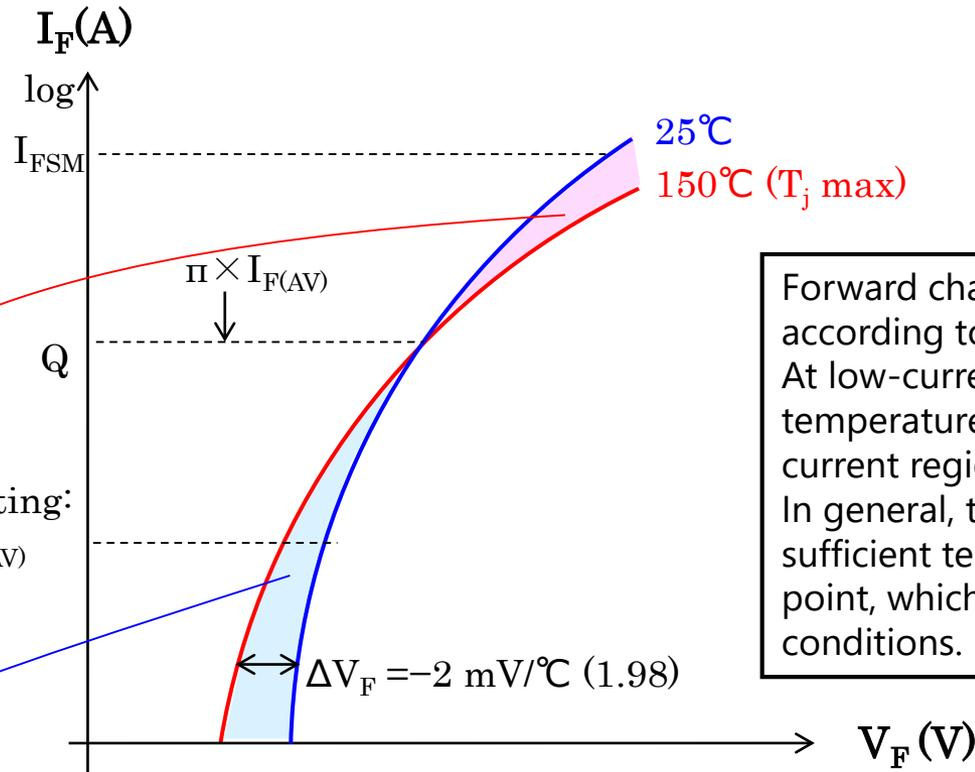
Forward characteristic of rectifier diode varies according to current level and temperature. At low-current region,  $V_F$  is low at high temperature, and the opposite is true at high-current region. In general, the diode should be used with a sufficient temperature margin below the Q point, which is the cross point of the above two conditions.
