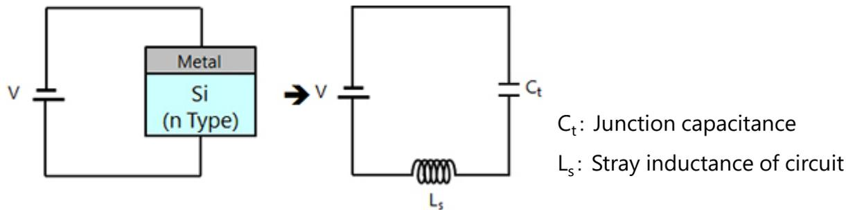
Fig. 2-10(a) Equivalent circuit when reverse voltage is applied to SBD
