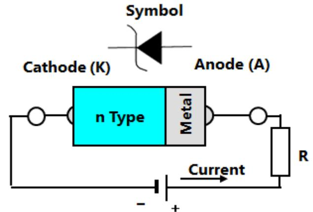
Fig. 2-9(a) Symbol and structure of Schottky barrier diode
